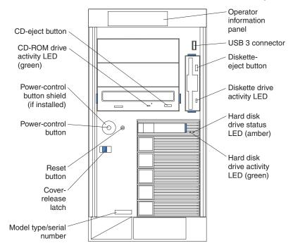
Note: The front bezel door is not shown so that the drive bays are visible.
