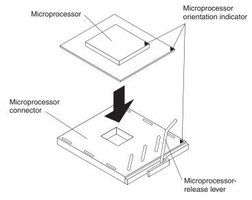
**Attention:** To avoid bending the pins on the microprocessor, do not use excessive force when pressing it into the socket.
