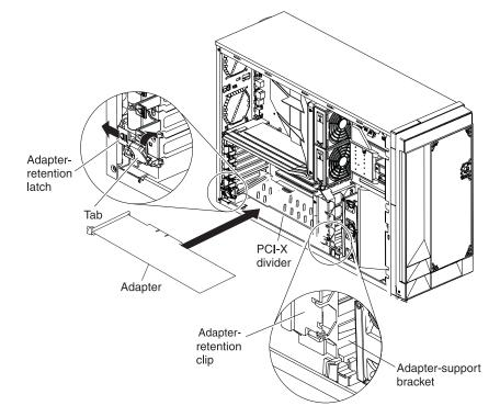
Complete the following steps to install a hot-plug PCI or PCI-X adapter:
