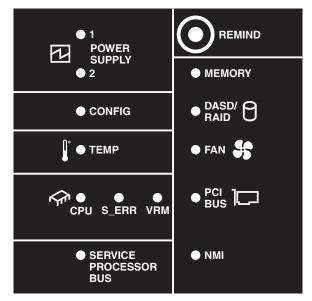
Use the remind button on the light path diagnostic panel to acknowledge that an error has occurred without taking further action. When you push the remind button the system error LED will flash every 2 seconds until the error is fixed. If another error occurs the system error LED will then stop flashing and return to a solid on state.
