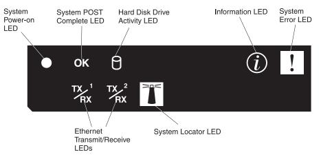
The following LEDs are on the operator information panel:
