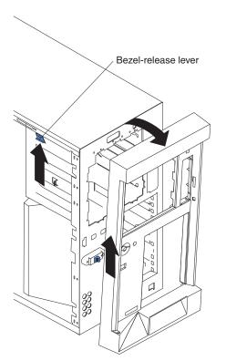
Complete the following steps to remove the bezel:
