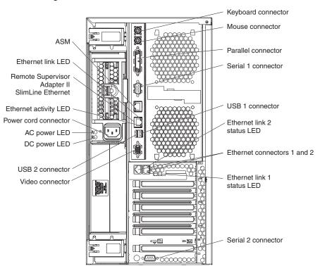
The following illustration shows the connectors and LEDs on the rear of the server.
