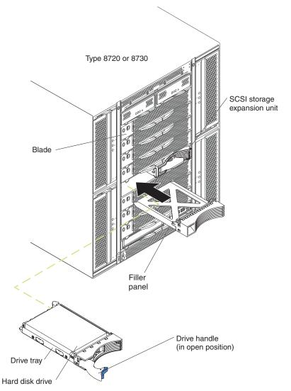
**Attention:** To maintain proper system cooling, do not operate the unit for more than 1 minute without either a hard disk drive or filler panel installed in each drive bay.
