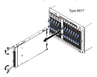
Note: You must remove the bezel assembly from the BladeCenter T unit before you can access the blade server. Firmly grip the blue touch points (at the top-left and top-right sides of the bezel) and forcefully pull forward, lifting the bezel up and away from the BladeCenter T unit. Carefully set the bezel assembly aside in a safe place.
