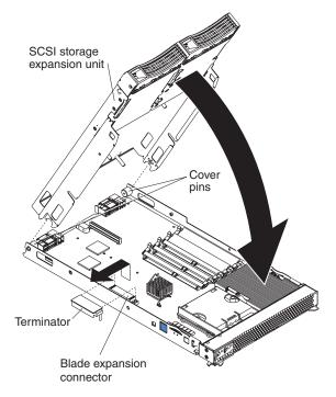
**Attention:** If installing a SCSI storage expansion unit on the BladeCenter HS40 Type 8839 blade server, then only install the compatible SCSI storage expansion units that do not have a shield, as shown in the following illustration.
