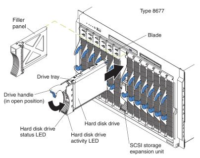
The following illustration shows how to install a SCSI hot-swap hard disk drive in the BladeCenter T unit.
