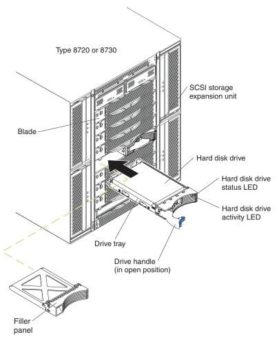
**Attention:** To maintain proper system cooling, do not operate the unit for more than 1 minute without either a hard disk drive or filler panel installed in each drive bay.
