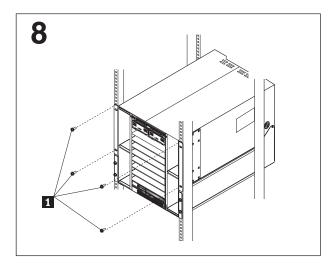
Install two M6 combination-head screws into each mounting bracket to secure the unit to the rack 1.
