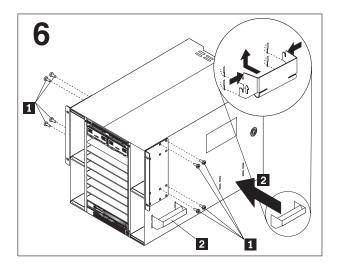
Attach the two mounting brackets to the sides of the unit by installing eight M4 flathead x + 8mm screws 1.
