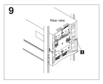
From the rear of the rack, secure the two captive screws, located in each blower bay, to the shelf brackets 1. Reinstall the blowers in the BladeCenter T unit. (See the *BladeCenter T Types 8720 and 8730 Installation and User's Guide* for installation procedures.)
