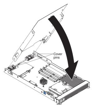
17. Pivot the cover to the closed position, as shown in the illustration, until it clicks into place.
