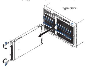
Note: You must remove the bezel assembly from the BladeCenter T unit before you can access the blade server. Firmly grip the blue touch points (at the top-left and top-right sides of the bezel) and forcefully pull forward, lifting the bezel up and away from the BladeCenter T unit. Carefully set the bezel assembly aside in a safe place. (See the BladeCenter T Types 8720 and 8730 Installation and User's Guide for detailed instructions about removing the bezel assembly.)
