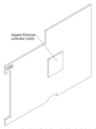
**Gigabit Ethernet controller (U25):** Each channel of the dual-channel Gigabit Ethernet controller on the I/O expansion card provides an output that is routed to a different I/O-module bay on the BladeCenter unit.
