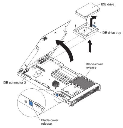
10. If an IDE drive is in IDE connector 2, remove the drive and tray (save the screws that secure the tray to the system board); otherwise, remove the two rear-board mounting screws (near IDE connector 2).
