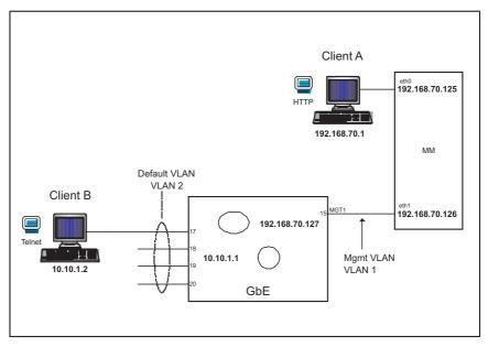
Client A manages the Gigabit Ethernet switch module through the default management-module configuration interface. The management module is always enabled and always a member of VLAN 1. VLAN 1 can never be disabled. You can always manage the Gigabit Ethernet switch module over this interface, provided that the IP addresses of the client, the management module, and the Gigabit Ethernet switch module are on the same subnet, as shown in the following table.
