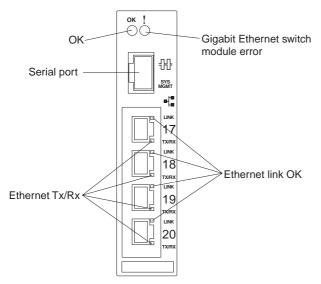
**OK:** This green LED is on the left side of the information panel, above the four external 10/100/1000 Mbps connectors. When this LED is lit, it indicates that the Gigabit Ethernet switch module has passed the power-on self-test (POST) with no critical faults and is operational.
