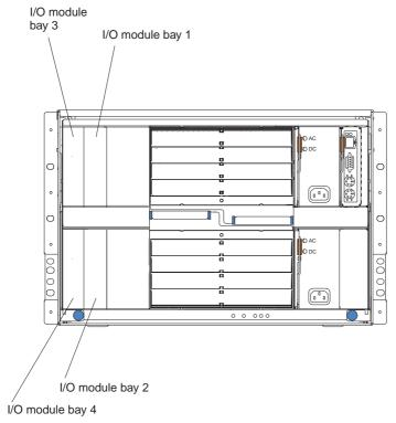
**Attention:** To maintain proper system cooling, each I/O-module bay must contain either a module or a filler module; each blade bay must contain either a blade or a filler blade.
