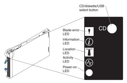
**Blade-error LED:** When this amber LED is lit, it indicates that a system error has occurred in the blade server.
