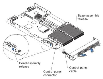
Complete the following steps to remove the blade-server bezel assembly:
