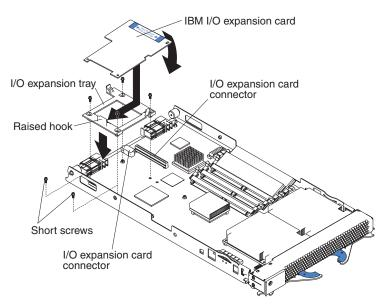
Complete the following steps to install an I/O expansion card:
