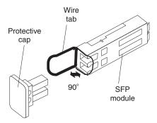
Figure 20. Unlocking an SFP module - wire tab
