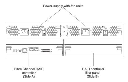
Figure 5. DS400 storage subsystem rear view
