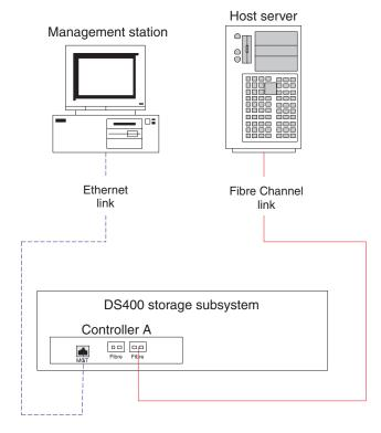
Figure 13. Single server, single storage subsystem configuration (DS400)
