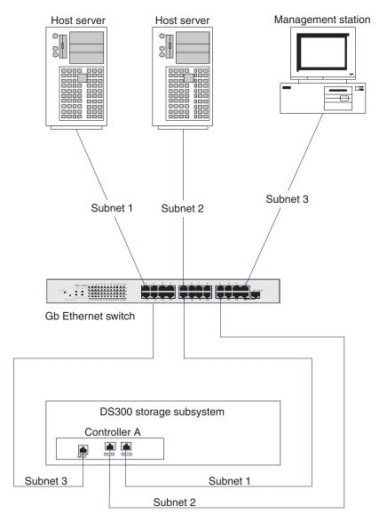
Figure 10. Single port, two-server configuration (DS300)
