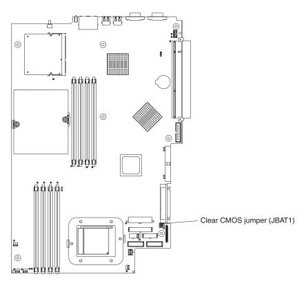
Attention: Before changing any switch settings or moving any jumpers, turn off the server; then, disconnect all power cords and external cables. See the safety information beginning on page v. Do not change settings or move jumpers on any system-board switch or jumper blocks that are not shown in this book.
