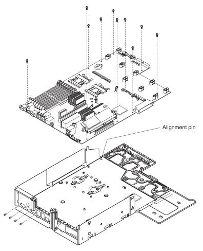
16. Align the replacement system board with the shuttle and replace the screws that were removed.
