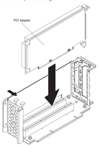
The following illustration shows how to install an adapter in the PCI riser-card cage.
