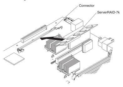
**Note:** If there is a gap between the card and the retaining clips, the card has not been properly installed. In this case, open the retaining clips and remove the card; then, reinsert the card.
