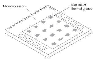
5. Use the thermal grease syringe to place 16 uniformly spaced dots of 0.01mL each on the top of the microprocessor.
