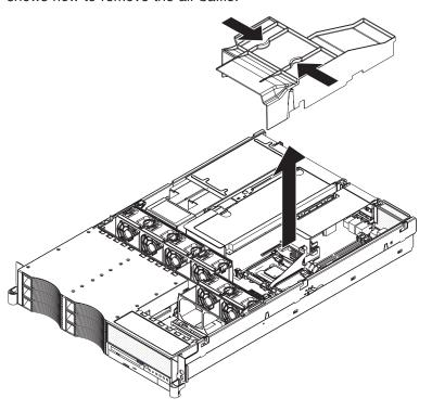
Complete the following steps to remove the air baffle:
