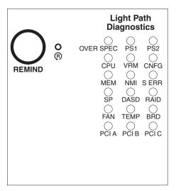
To acknowledge a system error but not take immediate action, press the remind button and place light path diagnostics in remind mode. When the server is in remind mode, the system-error LED on the front of the server flashes. If a new failure occurs, the system-error LED is lit again.
