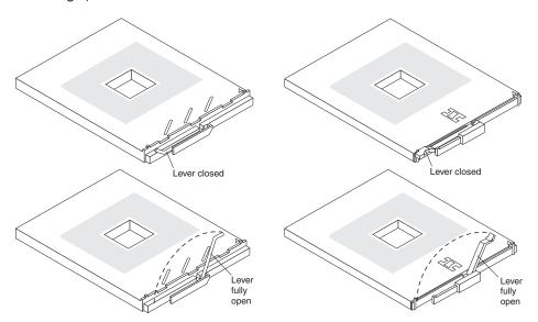
Attention: Do not use excessive force when removing the microprocessor form the socket.
