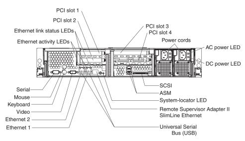
**Ethernet link status LEDs:** When these LEDs are lit, they indicate that there is an active link connection on the 10BASE-T, 100BASE-TX, or 1000BASE-TX interface for the Ethernet port.
