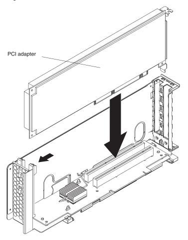
7. If you removed the PCI low-profile-card cage to install the adapter, press the PCI low-profile-card cage *firmly* into the connector until the retention latch locks.
