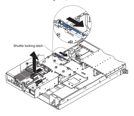
To install a shuttle with a preinstalled system board, slide the shuttle into the server and close the shuttle locking latch. Reverse the previous steps to replace the components that were removed. To remove the system board from the shuttle, continue with the next step.
