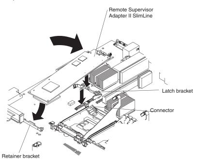
Slip the free end of the card under the tab on the retainer bracket; then, press the card in the connector and make sure that all tabs on the latch bracket secure the card in place.
