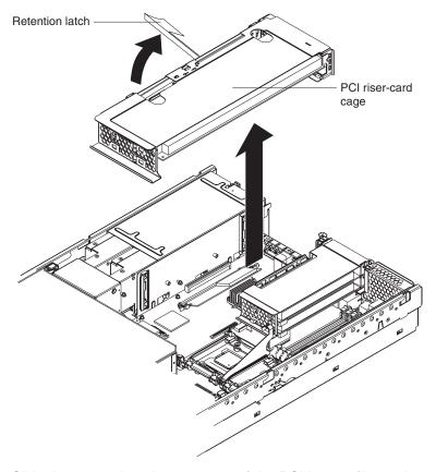
5. Slide the expansion-slot cover out of the PCI low-profile-card cage or PCI riser-card cage.
