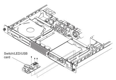
Complete the following steps to remove the Switch/LED/USB card.
