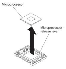
Complete the following steps to remove a microprocessor.
