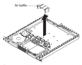
Complete the following steps to remove the air baffle.
