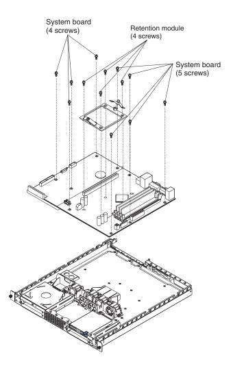
Complete the following steps to remove the system board.
