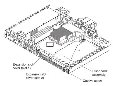
6. Remove the expansion-slot cover.
