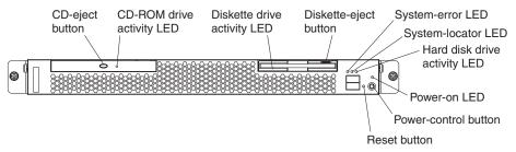
CD-eject button: Press this button to release a CD from the CD-ROM drive.
