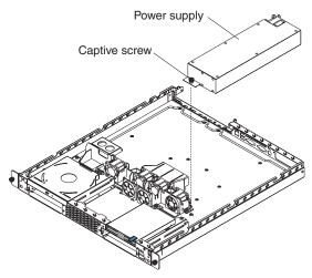
Complete the following steps to remove the power supply.
