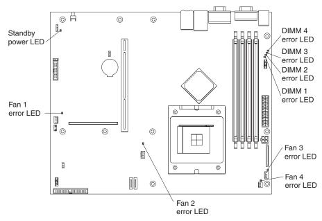
Each error LED is lit to indicate a problem with a specific component. After a problem is corrected, its LED will not be lit the next time the server is restarted; if the problem remains, the LED will be lit again.
