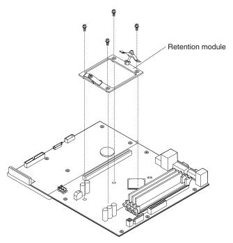
Complete the following steps to remove the retention module.
