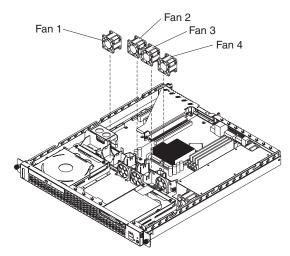
5. Position the replacement fan so that the airflow arrow on the side of the fan is pointing toward the rear of the server.
