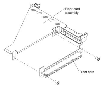
Complete the following steps to remove the PCI riser card.
