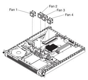
The server comes with six replaceable fans. Complete the following steps to replace a fan assembly.
