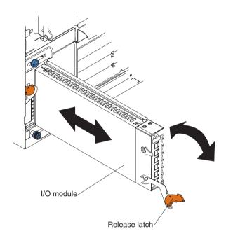
Complete the following steps to install an I/O module.
