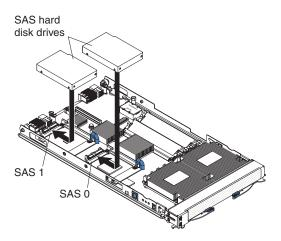
Note: Do not install a SAS hard disk drive in SAS connector 1 (J501) if you intend to also install an optional standard-form-factor expansion card. The standard-form-factor expansion card occupies the same area as the second hard disk drive.
