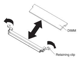
To install a DIMM, complete the following steps:
