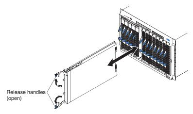
To install a blade server in a BladeCenter unit, complete the following steps.
