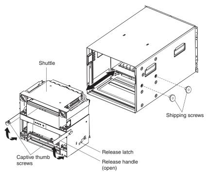
**Attention:** The BladeCenter unit comes with two shipping screws in each side of the chassis that help prevent damage to the shuttle during shipment. Make sure that these screws have been removed before attempting to remove the shuttle.
