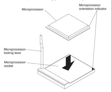
**Attention:** Make sure that the microprocessor is oriented and aligned correctly in the socket before you try to close the lever.
