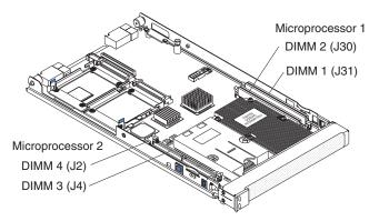
6. To remove a DIMM, repeat the following steps for each DIMM that you want to remove:
