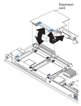
5. Gently pivot the wide end of the card out of the expansion card connectors; then, slide the notched end of the card out of the raised hook on the tray and lift the card out of the blade server.
