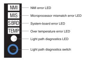
Note which LEDs are lit on the system board and the light path diagnostics panel. Using this information and the information in "Light path diagnostics LEDs" on page 42 can often provide enough information to diagnose the error.
