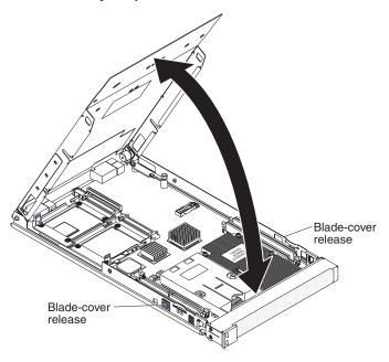
**Important:** The blade server cannot be inserted into the BladeCenter unit until the cover is installed and closed. Do not attempt to override this protection.
