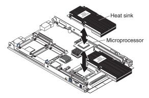
**Attention:** Do not use any tools or sharp objects to lift the locking lever on the microprocessor socket. Doing so might result in permanent damage to the system board.
