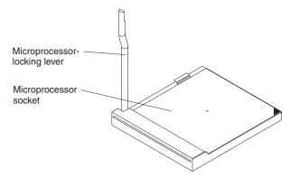
Avoid touching the components and gold pins on the microprocessor. Make sure that the microprocessor is completely and correctly seated in the socket. Incomplete insertion might cause damage to the system board or to the microprocessor. Touch the static-protective package that contains the replacement
