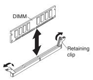
b. Turn the DIMM so that the DIMM keys align correctly with the connector on the system board.
