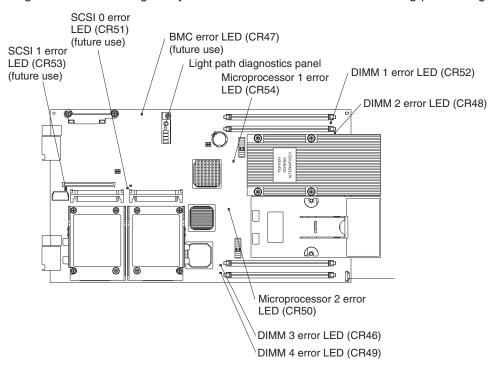
The following illustration shows the light path diagnostics panel on the system board.
