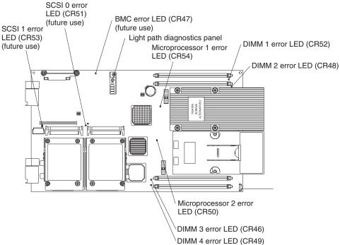
The following illustration shows LEDs on the light path diagnostics panel on the system board.
