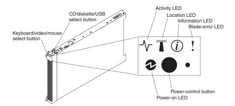
**Keyboard/video/mouse (KVM) select button:** Press this button to associate the shared BladeCenter unit keyboard port, video port, and mouse port with the blade server. The LED on this button flashes while the request is being processed then is lit when the ownership of the keyboard, video, and mouse has been transferred to the blade server. It can take approximately 20 seconds to switch the keyboard, video, and mouse control to the blade server.
