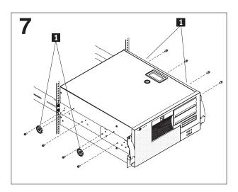
Use four M4 screws on each side of the system to secure the system to the rails; then, remove the rack-support wheels **1** and store them in a safe place.
