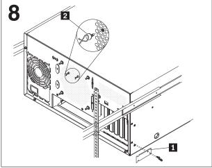
Use two M4 screws to install the cable-retainer bracket 1 on the right-rear of the system; then, install the cable clamps 2.
