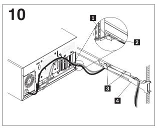
Use a cable strap 1 to attach all of the cables to the cable-retainer bracket 2 on the cable-management arm 4.
