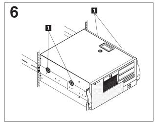
Fully extend the slide rails out of the rack cabinet; then, lift the system above the rails and rest the rack-support wheels 1 on the slide rails.
