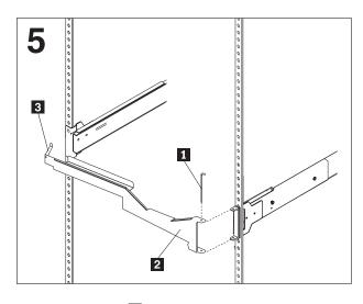
Use the hinge pin 1 to attach the cable-management arm **2** to the hinge bracket.
