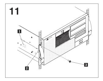
Press in on the safety latch 1 and slide the system into the rack cabinet until the release latches 2 snap into place; then, insert the M6 screws 3 through the release-latch-bracket assembly.
