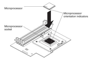
14. Close the microprocessor-release lever to secure the microprocessor.
