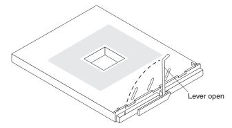
**Attention:** You must make sure that the locking lever on the microprocessor socket is in the fully open position before you insert the microprocessor in the socket. Failure to do so might result in permanent damage to the microprocessor, microprocessor socket, and system board.
