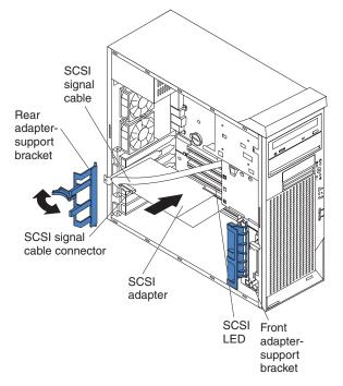
3. Complete the installation of the optional SCSI adapter.
