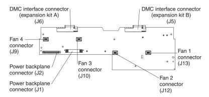
Figure 9. Drawer management controller internal connectors
