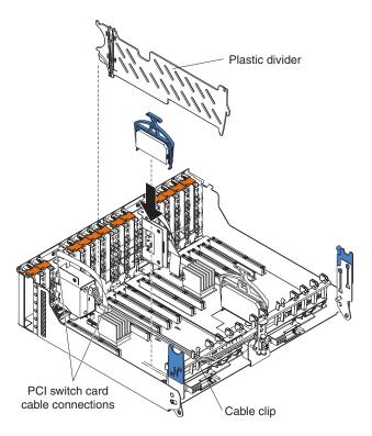
Figure 21. Installing a PCI-X expansion board ribbon power cables
