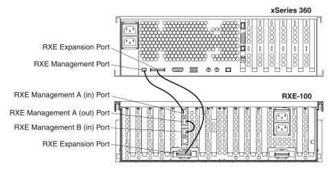
Figure 28. Server controlling two systems in the enclosure
