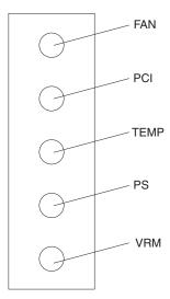
These LEDs can indicate a problem with a single component, or a problem with one of several similar components. In the latter case, to isolate the specific failing component, remove the server top cover and look for a lit LED on the PCI expansion board.
