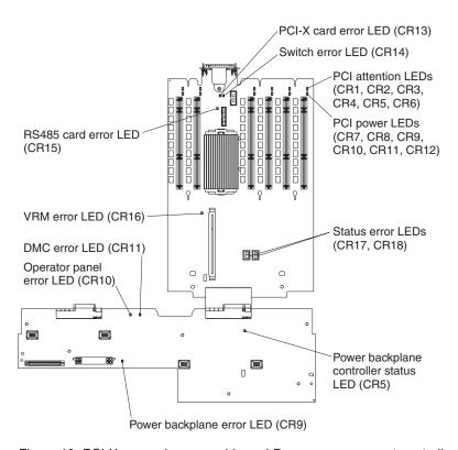
Figure 12. PCI-X expansion assembly and Drawer management controller LEDs
