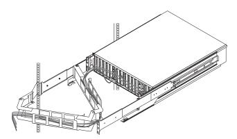
Figure 29. Routing the cables
