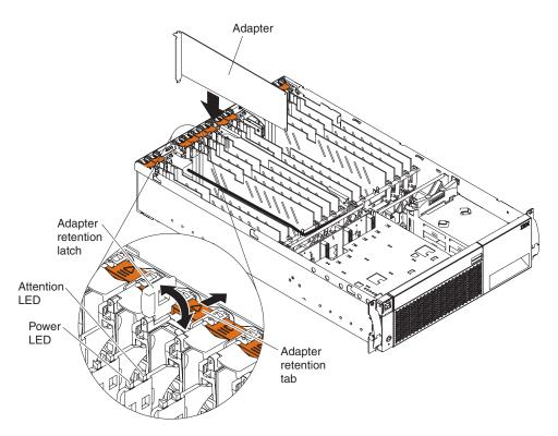
Figure 15. Installing an adapter
