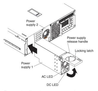
Figure 22. Installing a hot-swap power supply
