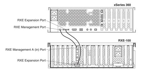
Figure 27. Server controlling one system in the enclosure
