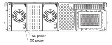
Figure 1. Front panel of enclosure
