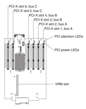
Figure 14. Hot-plug PCI slot locations
