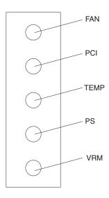
Figure 11. Diagnostic panel LEDs
