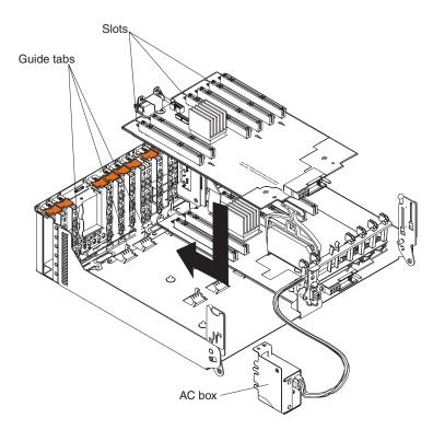
Figure 18. Installing a PCI-X expansion board
