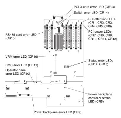
Figure 6. PCI-X expansion assembly LEDs
