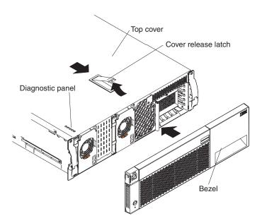
Figure 25. Installing the enclosure top cover and bezel
