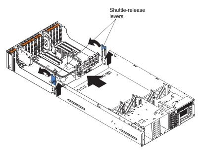
Figure 17. Sliding the shuttle release levers toward the rear
