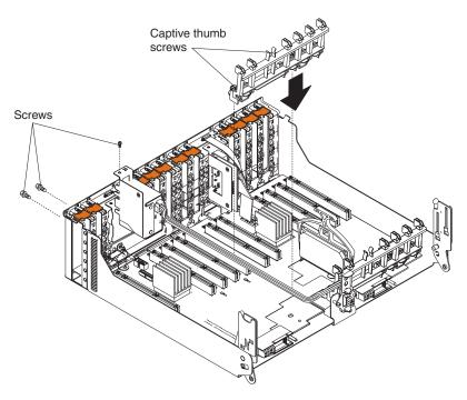
Figure 19. Installing the new rear support PCI holder
