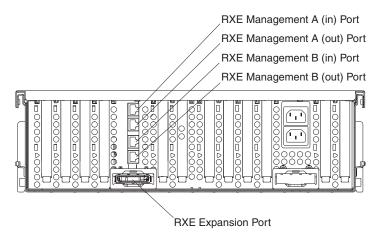
Figure 26. Input/output ports
