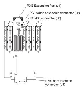
Figure 10. PCI-X expansion assembly external and internal connectors
