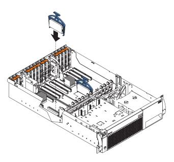
Figure 24. Replacing a VRM
