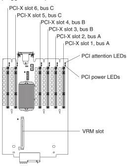
Figure 8. PCI-X expansion assembly components connectors
