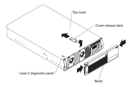
Figure 13. Removing the top cover and bezel
