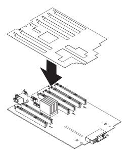
Figure 16. Installing the insulation shield
