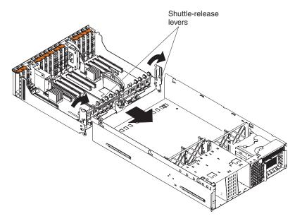
Figure 20. Sliding the shuttle release levers toward the front
