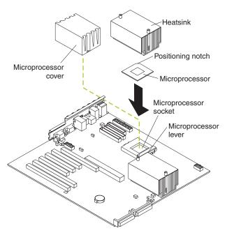
16. When you tighten the screws to secure the heatsink, alternate between the two screws. That is, tighten one screw a little then tighten the other screw a little. Continue switching between the screws until the heatsink is secured to the microprocessor. Alternating the tightening of the screws can help prevent damage to the microprocessor.
