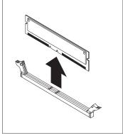
8. Store the RIMM or C-RIMM in a static-protective package. Do not discard or lose this part. It might be needed later if you change the memory configuration.
