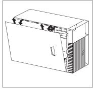
7. Lift the lever at the top of the chassis and pull the front bezel from the front of the computer. You might need to move the computer closer to the edge of the desk to completely rotate the bezel down to remove it.
