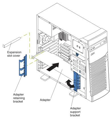
Complete the following steps to install an adapter:
