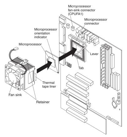
Complete the following steps to remove a microprocessor.
