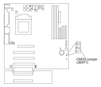
The default position is a jumper installed on pins 1 and 2. Before you change the position of this jumper, you *must* turn off the server and peripheral devices, and disconnect all external cables and power cords. Remove the cover and then move the jumper to pins 2 and 3.
