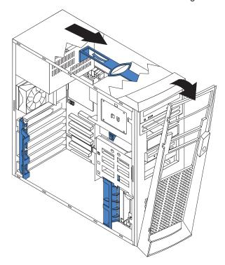
Complete the following steps to remove the bezel:
