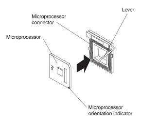
**Attention:** Do not use excessive force when pressing the microprocessor into the connector.
