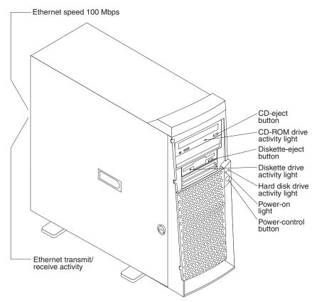
CD-eject button: Push this button to open the CD tray to insert or remove a CD.
