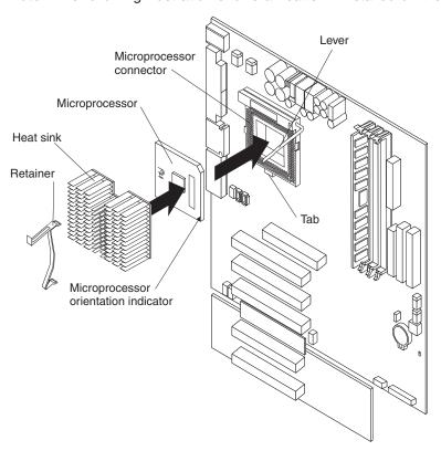
**Note:** This illustration shows the fan sink installed on the microprocessor.
