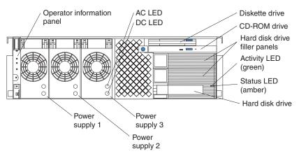
**Operator information panel:** This panel, also known as the front LED panel, contains controls, indicators, and one of the three USB ports. See "Operator information panel" on page 9 for details.
