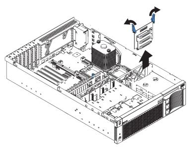
2. Remove from the server the metal mounting plate that holds the Lightpath Diagnostic card and the hot-swap drive backplane as described at step 2 on page 105 through step 4 on page 106 of "Hot-swap drive backplane" on page 105.
