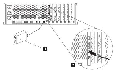
2. Connect one or two Ethernet cables of the appropriate type (Category 5 is recommended) to the other end of the ASM Interconnect module.
