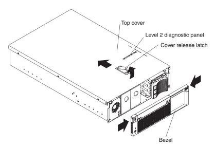
1. Lift the plastic cover-release latch on the top cover.
