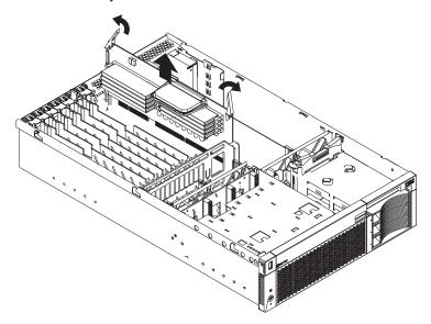
When installing additional DIMMs, determine the DIMM slots into which you will install them. You must populate the slots in pairs, one DIMM in each column, proceeding from top to bottom. Use only 2.5 V, 184-pin, PC1600, DDR registered synchronous dynamic random-access memory (SDRAM) with error
