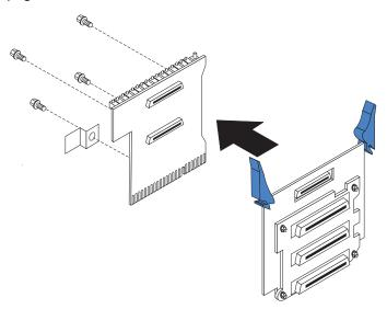
3. Set the metal plate containing the hot-swap drive backplane and the Lightpath Diagnostic card on a static-free surface and remove the 4 screws that secure the Lightpath Diagnostic card to the plate, detaching any Lightpath Diagnostic card cables.
