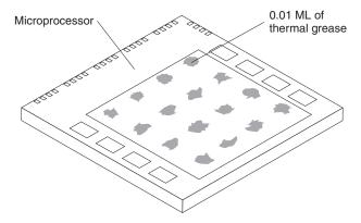
6. Install the heatsink onto the microprocessor as described in the documentation that comes with the computer or server.
