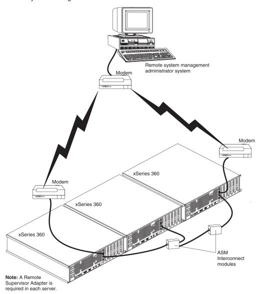
**Note:** The ASM Interconnect module is connected to the RS485 port on the back panel of the Remote Supervisor Adapter in each server.
