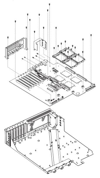
6. Remove the other 18 screws that secure the system board to the shuttle, and put the screws in a safe place.
