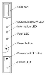
**USB port:** This port enables you to attach a USB device to the front of the server.
