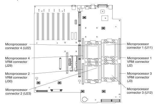
Complete the following steps to install a microprocessor:
