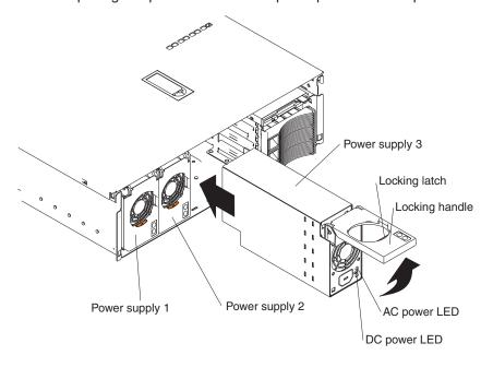
**Note:** The power supplies are numbered from left to right (1 to 3) as viewed from the front of the server. Power supplies do not have to be installed in a particular sequence.
