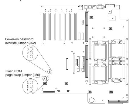
Changing the position of the jumper on J52 bypasses the power-on password check *if* the jumper has been moved since the server was last powered on. You must move the jumper back to the default position after the password is overridden. The default position is pins 1 and 2.
