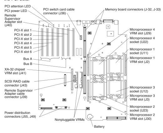
The following illustration shows the location of the internal connectors on the system board.
