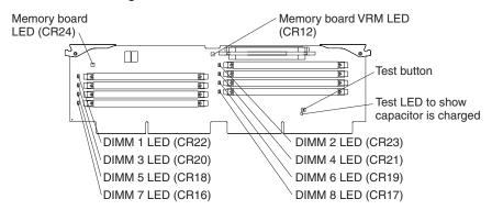
If the DIMM LED is not visible with the memory board in place, after removing the memory board you can press the Test button on the board to relight the failing DIMM's LED. If no DIMM has failed, pressing the Test button lights the Test LED.
