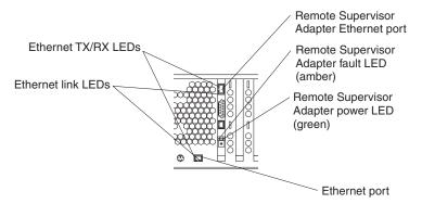
**Ethernet Link LEDs:** These LEDs (one for the Remote Supervisor Adapter, one for the network) indicate that the related Ethernet link is operational.
