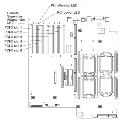
2. Determine which PCI-X expansion slot you will use, slide its orange adapter-retention tab toward the rear of the server, and lift the adapter-retention
