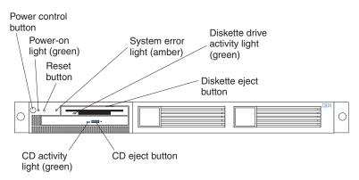
Power-control button: Press this button to manually turn the server on or off.
