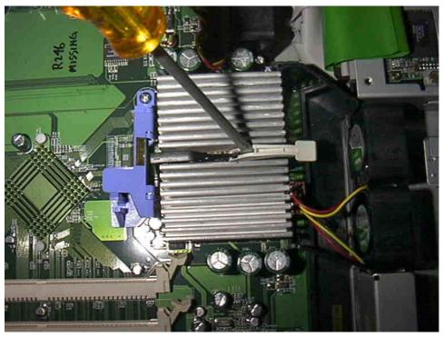
If the handle breaks, remove the handle by placing a screw driver in between both sides of the handle as in the picture above, and twist the screw driver to break off the handle to relieve the pressure from the clip to the heat sink, as in the picture below.
