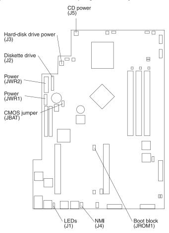
The following illustration identifies the jumpers on the system board.
