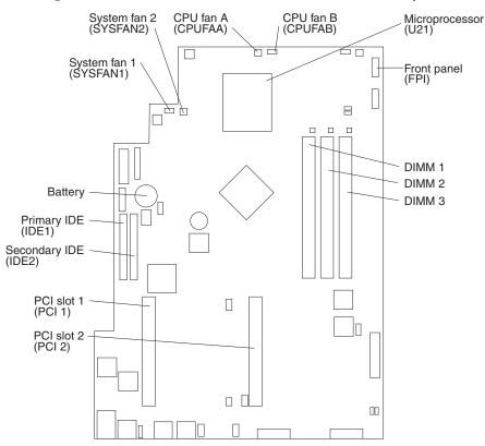
The following illustration identifies the internal connectors on the system board.
