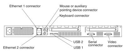
To effectively manage the cables on this server, keep groups of cables secured together, and do not run cables across the back of the server.
