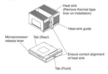
b. Align and place the heat sink on the top of the microprocessor.
