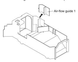
a. Remove the air-flow guide 1 (external) from the air-baffle assembly by rotating the guide in a back and forth motion.
