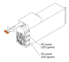
**AC Power Light:** This light provides status information about the power supply. During normal operation, both the AC and DC Power lights are on. For any other combination of lights, see "Power supply LED errors" on page 92.
