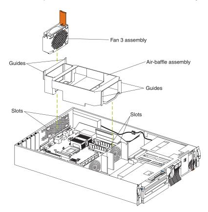
9. Reinstall the fan 3 assembly and make sure the fan is fully seated into the connector.
