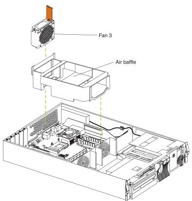
4. Remove the air baffle by grasping it at the sides and lifting it from the server.
