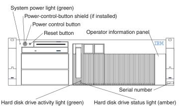
**System Power Light:** When this green light is on, system power is present in the server. When this light flashes, the server is in standby mode (the system power supply is turned off and AC current is present). When this light is off, either a power supply, AC power, or a light has failed.
