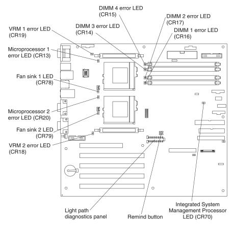
**Light Path Diagnostics panel**The Light Path Diagnostics LEDs are described in the following table.
