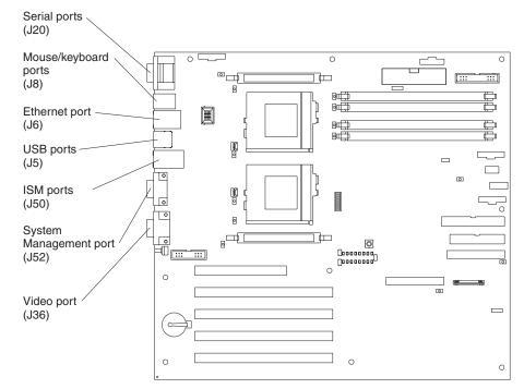
Future releases of the Integrated System Management (ISM) firmware code will enable the Integrated System Management processor to send or forward alerts to IBM system management adapters using the ISM ports.
