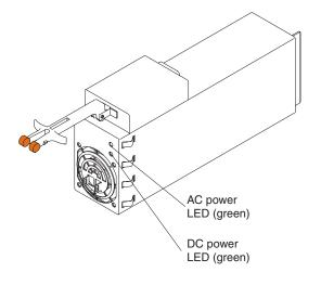
**AC power light:** This green light on the power supply (behind the bezel) provides status information about the power supply. During normal operation, both the ac and dc power lights are on. For any other combination of lights, see "Power-supply LEDs" on page 106.
