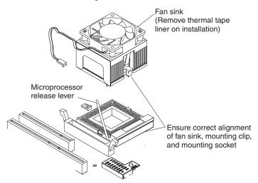
Make sure the fan sink guide fits between the processor and the processor socket.
