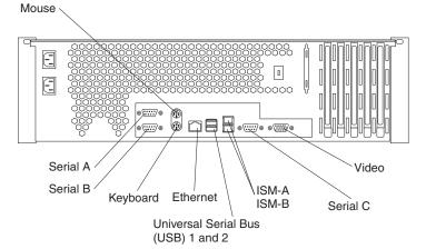
Future releases of the Integrated System Management (ISM) firmware code will enable the Integrated System Management processor to communicate using a modem and the dedicated Serial C port.
