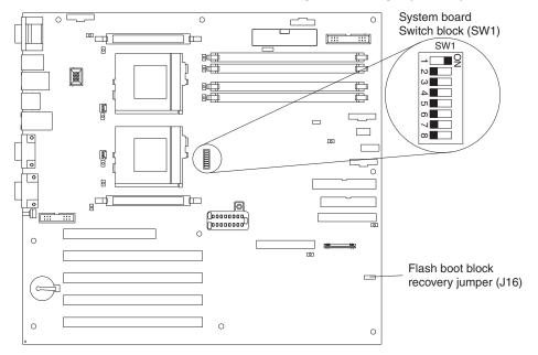
**Note:** Any jumper blocks on the system board that are not shown in the illustration are reserved.
