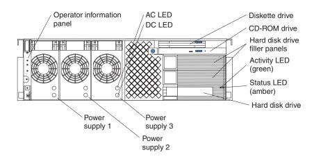
**Operator information panel:** This panel, also known as the front LED panel, contains controls, indicators, and one of the three USB ports. See "Operator information panel" on page 27 for details.
