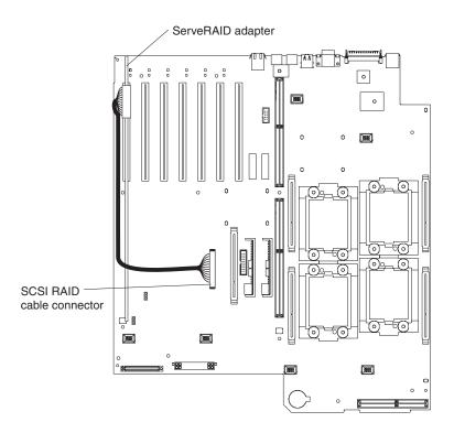
Route the cable along the surface of the system board toward the front of the server, then to the right under the adapters and dividers; then plug it into the SCSI RAID cable connector (J43) on the system board.
