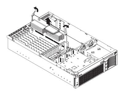
4. When installing additional DIMMs, determine the DIMM slots into which you will install them. You must populate the slots in pairs, one DIMM in each column, proceeding from top to bottom. Use only 2.5 V, 184-pin, PC1600, DDR registered synchronous dynamic random-access memory (SDRAM) with error correcting code (ECC).
