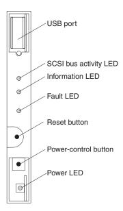
**USB port:** This port enables you to attach a USB device to the front of the server.
