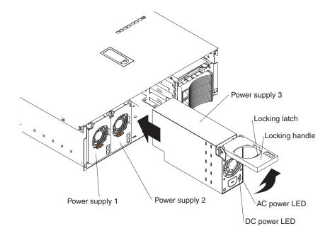
**Note:** The power supplies are numbered from left to right (1 to 3) as viewed from the front of the server. Power supplies do not have to be installed in a particular sequence.
