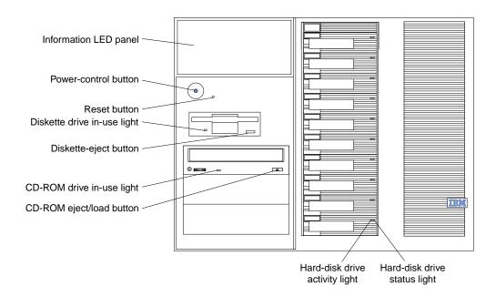
Hard-disk drive status light: Each hot-swap drive has a status light. When this amber light is on continuously, the drive has failed. If an optional IBM ServeRAID™ adapter is installed in the server, when the light flashes slowly (one flash per second), the drive is being rebuilt. When the light flashes rapidly (three flashes per second), the controller is identifying the drive.
