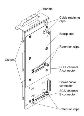
9. Attach one end of the SCSI cable to the selected internal SCSI channel connector on the ServeRAID adapter. Make sure that the other end of the SCSI cable is attached to the appropriate channel connector on the SCSI backplane.
