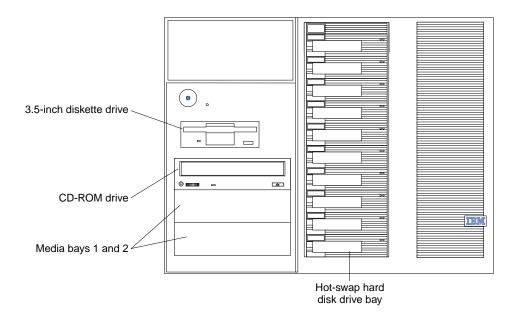
Each hot-swap drive has two indicator lights on the front of the server. If the amber hard-disk status light for a drive is lit continuously, that individual drive is faulty and needs to be replaced. When the hard-disk status light indicates a drive fault, you can replace a hot-swap drive without turning off the server.
