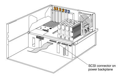
12. Slide the hot-swap hard disk drives back into place in the drive bays. If you need to install additional hot-swap drives, do so now (see "Installing a hot-swap hard disk drive" on page 62). You can connect a maximum of 10 hard disk drives to the SCSI backplane.
