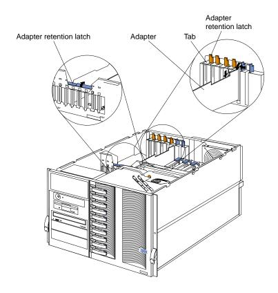
To install a non-hot-plug PCI adapter:
