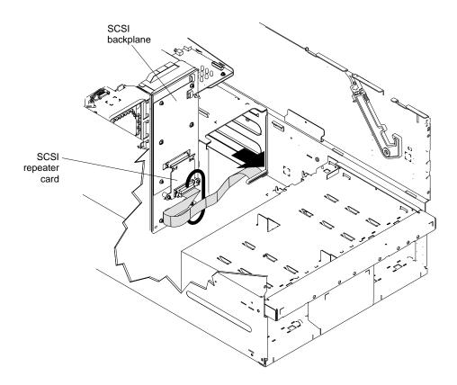
e. Make sure that the other end of the SCSI cable is attached to the power backplane located on the rear of the shuttle.
