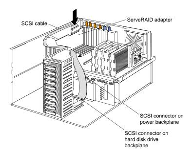
10. If you are connecting to two SCSI channels, repeat step 8 on page 49 and step 9 on page 50 for the second channel on the SCSI backplane. The following illustration is a top-down view that shows how to route two SCSI cables to the ServeRAID adapter in PCI slot 1.
