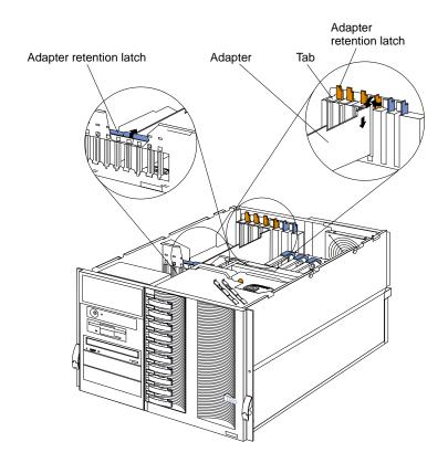
To install a hot-plug PCI adapter:
