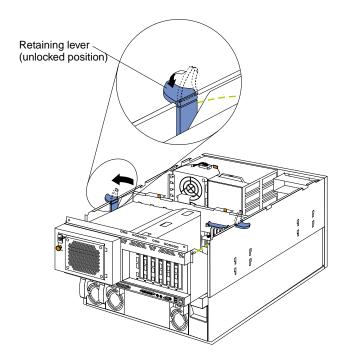
c. Slide the shuttle toward the rear of the server until it stops.
