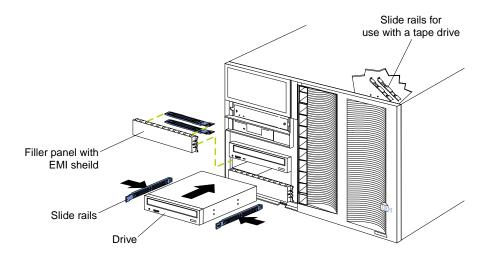
Choose the bay in which you want to install the drive. Also, check the instructions that come with the drive to see if you need to set any switches or jumpers on the drive.
