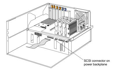
8. Route one end of the SCSI cable through the cable retaining clips on the SCSI backplane.
