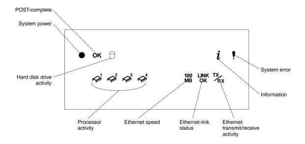
**System error light:** This amber light is on when a system error occurs. A light on the diagnostics LED panel will also be on to further isolate the error. (For more information, see "Diagnostic panel LEDs" on page 126.)
