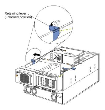
Slide the shuttle toward the rear of the server until it stops.
