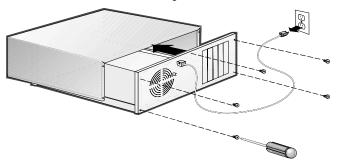
**3** Locate an unused 64-bit PCI/PCI-X expansion slot and remove the expansion slot cover. If the computer does not have a 64-bit slot, you can install the card in a 32-bit PCI slot. The Adaptec SCSI Card 29320ALP supports both 5V and 3.3V 64-bit slots. (The expansion slot must be compliant with PCI Rev. 2.2 or PCI-X Rev. 1.0 and must support Bus Mastering.) Save the slot cover screw for use in Step 4.
