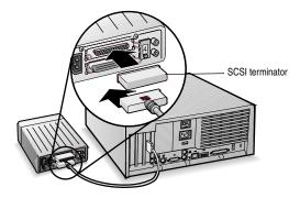
**3** Connect the other external SCSI devices by linking each device to the previous one, as shown below. Terminate only the device at the end of the chain.
