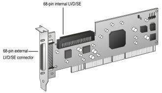
Although the Adaptec SCSI Card 29320ALP is a 64-bit PCI/PCI-X card, it also works in a 32-bit PCI slot. When installed in a 32-bit PCI slot, the card automatically runs in the slower 32-bit mode.
