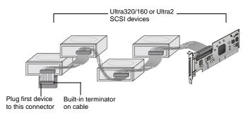
**Note:** Internal Ultra320/160 and Ultra2 SCSI devices come from the factory with termination disabled and cannot be changed. Proper termination is provided by the terminator at the end of the LVD SCSI cable.
