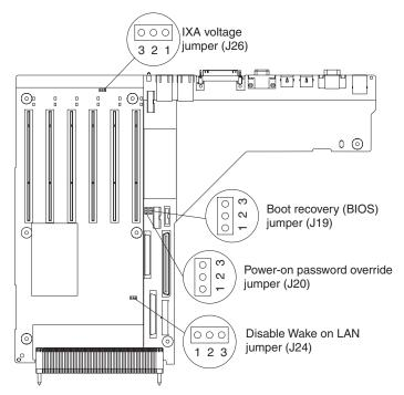
While the server is turned off, move the jumper on J20 from pins 1 and 2 to pins 2 and 3. You can then start the Configuration/Setup Utility program and reset the power-on password. After you reset the password, turn off the server again and move the jumper back to pins 1 and 2.
