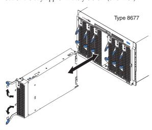
Note: You must remove the bezel assembly from the BladeCenter T unit before you can access the blade server. Firmly grip the blue touch points (at the top-left and top-right sides of the bezel) and forcefully pull forward, lifting the bezel up and away from the BladeCenter T unit. Carefully set the bezel assembly aside in a safe place. (See the BladeCenter T Types 8720 and 8730 Installation and User's Guide for detailed instructions about removing the bezel assembly.)
