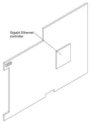
**Gigabit Ethernet controller:** Each channel of the dual-channel Gigabit Ethernet controller on the I/O expansion card provides an output that is routed to a different I/O-module bay on the BladeCenter unit.
