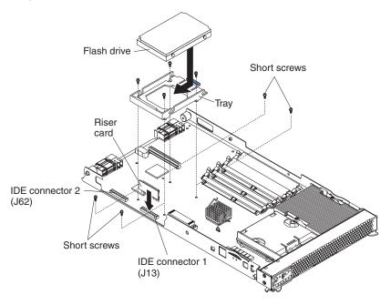
5. Place the flash drive tray from the option kit over the riser card as shown, aligning the tray with the screw holes on the system board. Two of the screw holes have screws in them.
