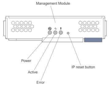
Management-module LEDs: These LEDs provide status information about the management module and remote management connection.
