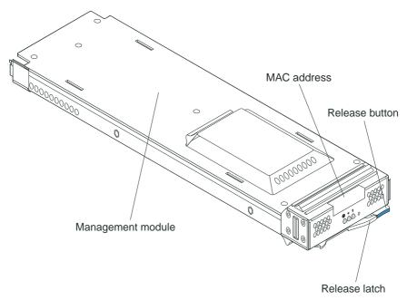
The IBM @server BladeCenter T Management Module is a hot-swap unit that is installed into the front of the BladeCenter T unit. The module contains the video compression boards.
