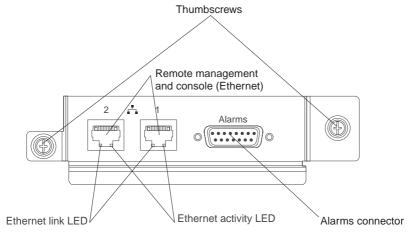
**LAN-module LEDs:** These LEDs provide status information about the LAN connection:
