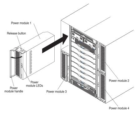
**Attention:** To help ensure proper cooling and system reliability, make sure that you replace a removed power module within 1 minute.
