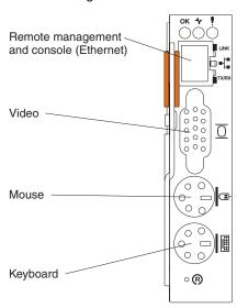
**Note:** There is no internal connections between the input/output connectors on the management modules when two are installed in the BladeCenter unit. See the *IBM BladeCenter Management Module Installation Guide* for information about how to cable two management modules to support the redundant management module interface requirements of your installation.
