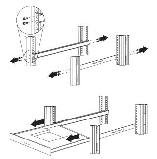
To remove the tray from the side rails, pull up on the left rail tab and push down on the right rail tab.
