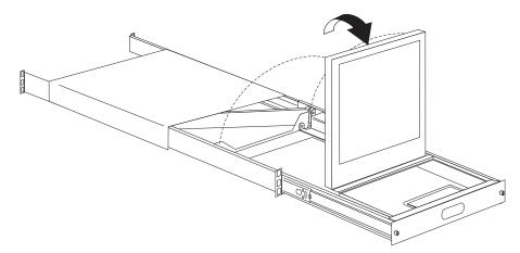
4. To remove the cable cover from the tray, remove the cable-cover screw; then, slide the cover toward the front of the tray until the tab on the tray can fit through the slot on the cover. Lift the cable cover from the tray and set it aside
