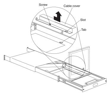
5. Ensure that the keyboard and mouse cable is routed through the slots on the bottom of the keyboard.
