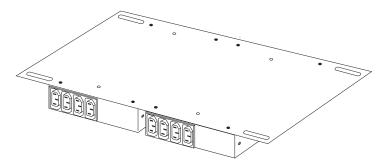
Figure 63. Installing a second Rack PDU
