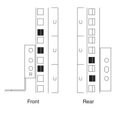
**Note:** Use clip nuts if your rack has circular holes. If your rack has square holes, you can use the rack-insertion tool or a flat-blade screwdriver to install cage nuts.
