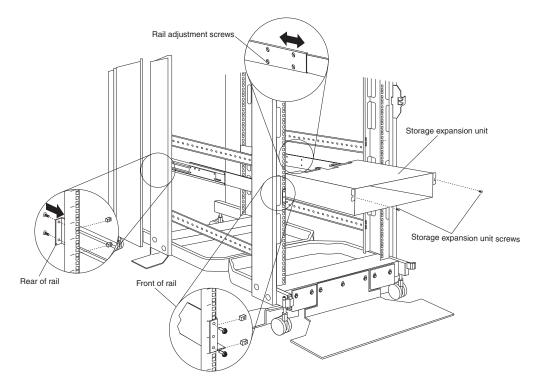
Figure 33. Installing a storage expansion unit
