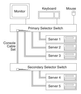
Figure 77. Multiple selector switch
