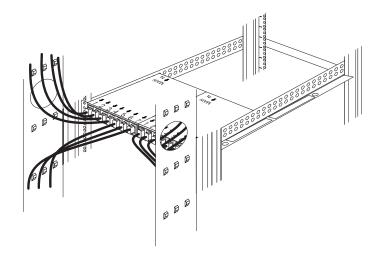
Figure 53. Connecting and routing other power cables to the outlets
