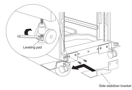
Figure 6. Lowering the NetBAY42 leveling pads and installing the side stabilizer brackets
