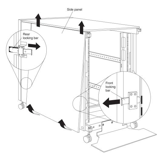
Figure 8. Removing the NetBAY25 side panels
