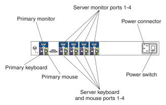
The 2x8 Console Switch allows you to connect up to eight servers to a primary and secondary monitor, mouse, and keyboard. Port **A** is located on the rear of the console switch and is where you connect your primary monitor, mouse, and keyboard. Port **B** is located on the front of the console switch and is where you connect your secondary monitor, mouse, and keyboard. Ports **1** through **8** are where you connect each of your servers.
