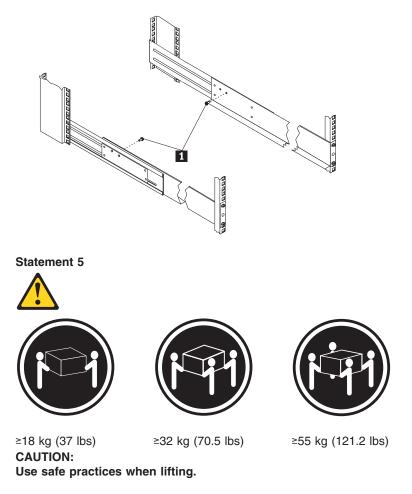
7. Slide the expansion unit into the rack, and insert the M6 screws 1. Do not overtighten the M6 1 screws.
