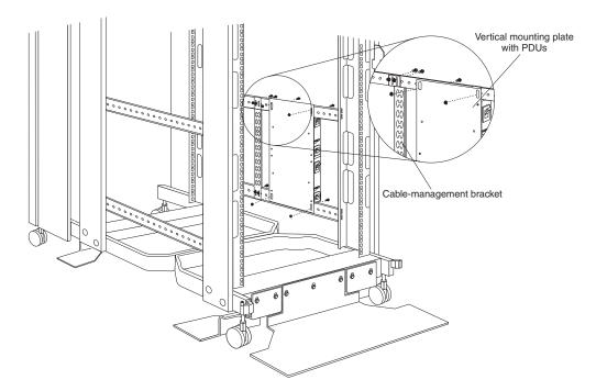
Figure 31. Installing a PDU vertically in a rack cabinet
