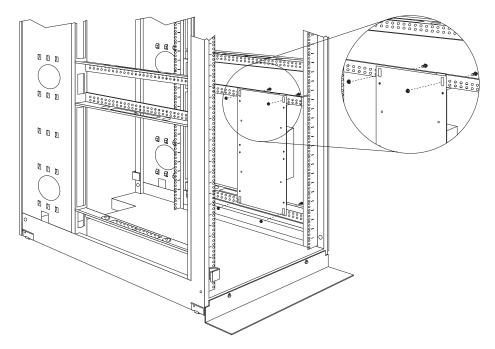
Figure 55. Installing the vertical mounting plate
