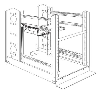
Figure 52. Connecting and routing the line cord
