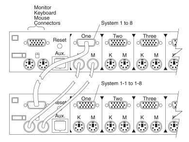
One eight-port primary selector switch can accommodate up to eight secondary selector switches which can then support up to 64 servers.
