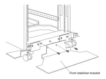
Figure 7. Installing the NetBAY42 front stabilizer bracket
