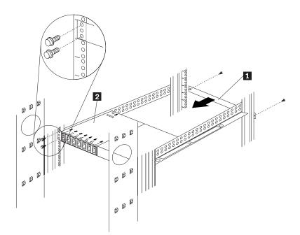
Figure 47. Installing the Rack PDU and the blank filler panel
