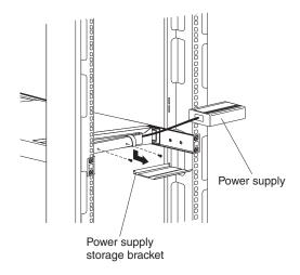
3. To remove the power supply storage bracket from the cable-management arm, remove the two screws and pull the bracket away from the arm. Store the parts in a safe place for possible future use.
