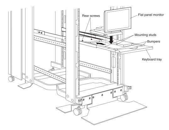
Figure 39. Installing a flat panel monitor rack mount kit
