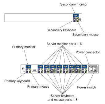
You can connect multiple console switches to each other in a tiered configuration. If you use a 1x4 Console Switch as the primary switch, you can connect up to four additional console switches and 32 servers. If you use a 2x8 Console Switch as the primary switch, you can connect up to eight console switches and 64 servers. The user interface of the primary switch will control all of the console switches in the tier.
