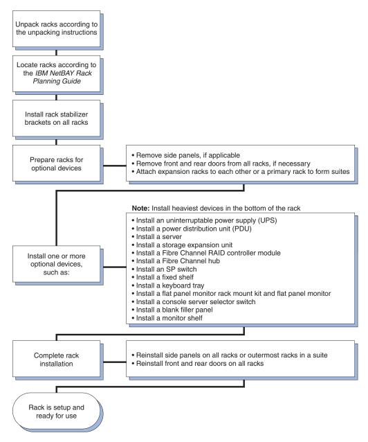
Figure 1. Installing the rack cabinet and devices overview
