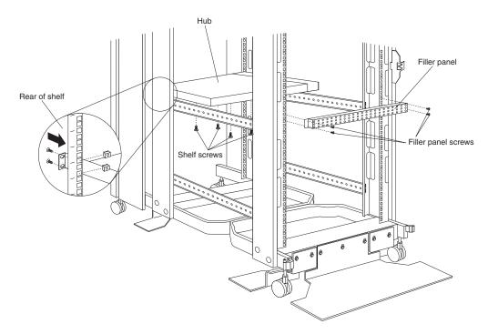
Figure 35. Installing a Fibre Channel hub
