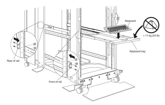
Figure 38. Installing a keyboard tray and keyboard
