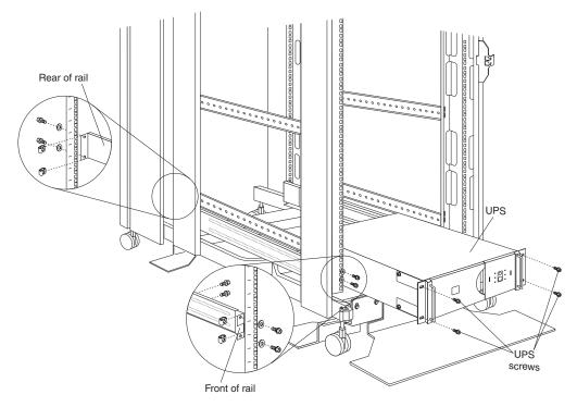
Figure 28. Installing a UPS
