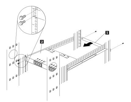
Figure 68. Installing the Rack PDUs and the blank filler panel
