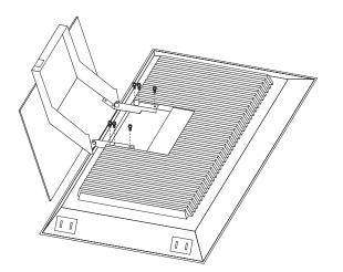
Figure 80. Removing the existing monitor stand from the monitor
