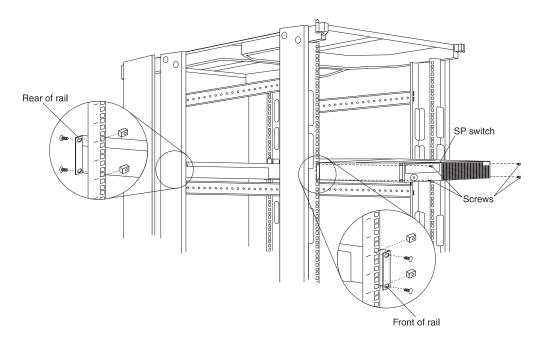
Figure 36. Installing an SP switch
