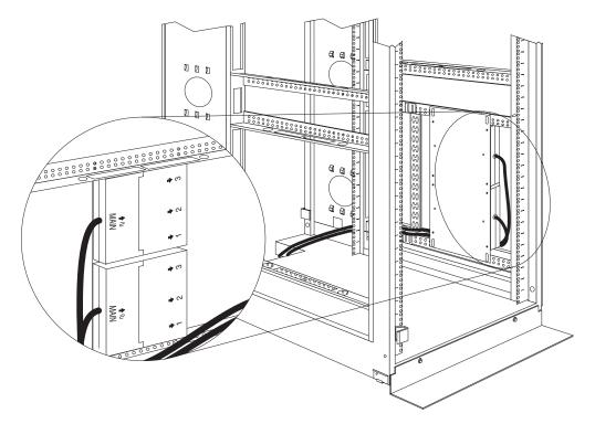
Figure 60. Routing the fixed line cords
