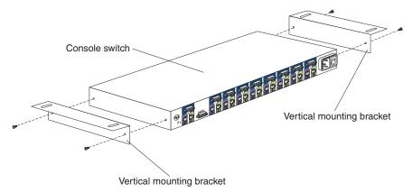
3. Hold the console switch against the side braces, with the rear of the console switch facing the back of your rack cabinet; then, use four M6 screws and nuts
