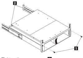
8. Tighten the rear screws 2.
