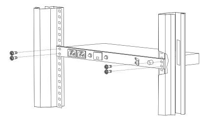
Figure 30. Power distribution horizontal installation
