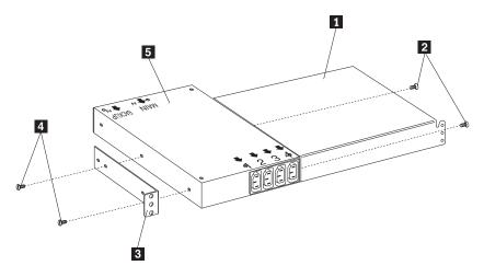
Figure 65. Installing the mounting brackets for a single device
