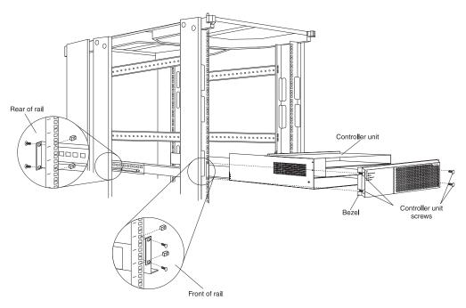
Figure 34. Installing a Fibre Channel RAID controller unit
