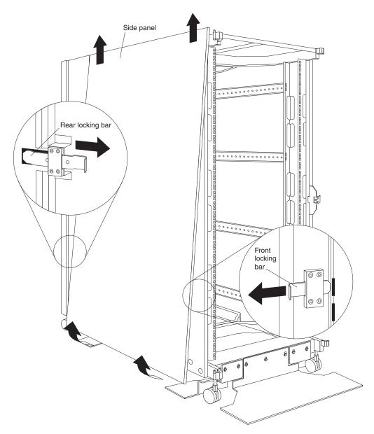
Figure 10. Removing the NetBAY42 side panels
