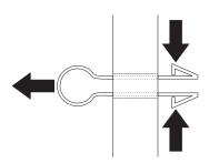
Figure 79. Removing the plastic cable clamp
