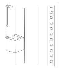
4. Remove the screw and nut that holds the hinge bracket **1** in place; then, move the hinge bracket 2 three mounting spaces downward and reinstall it at the new center location.
