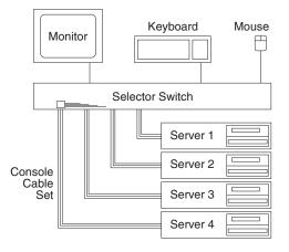
Figure 76. Single selector switch
