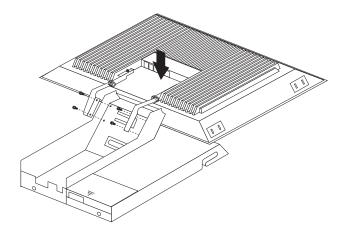
Figure 83. Installing the monitor on the new monitor stand
