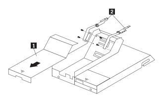
Figure 81. Removing the hinges from the new monitor stand
