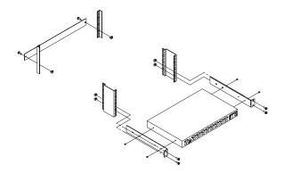
Figure 75. Selector switch rear of rack with blank panel front of rack
