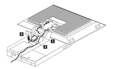
Figure 85. Storing the power supply and routing cables
