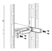
15. Install the screw that attaches the cable-management arm to the left slide-rail bracket; then, tighten all four slide-rail-adjustment screws.
