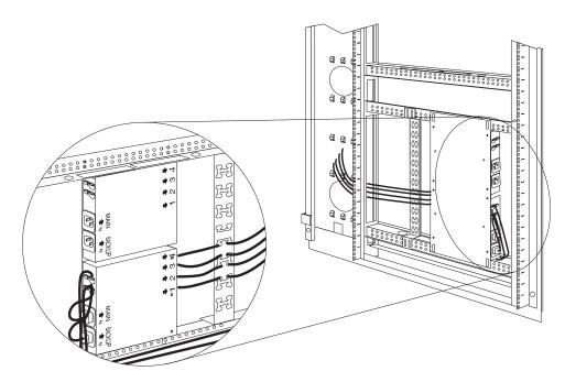
Figure 70. Connecting and routing other power cables to the outlets
