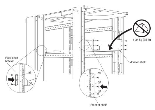
Figure 40. Installing a monitor shelf
