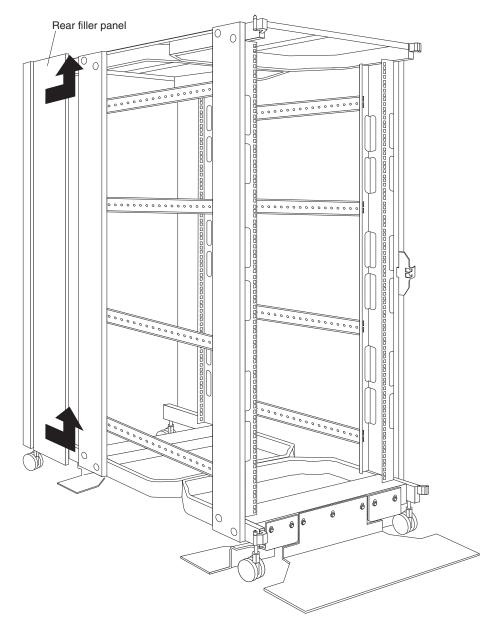
Figure 11. Removing the NetBAY42 rear filler panels
