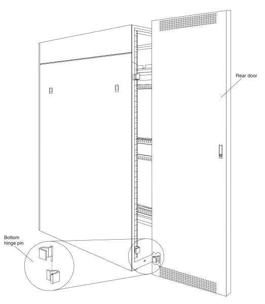
Figure 21. Removing a rear door from the rack cabinet
