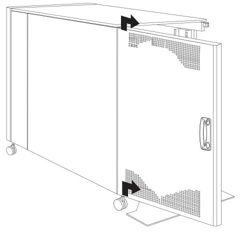
Figure 12. Removing a front door from the NetBAY25 rack cabinet
