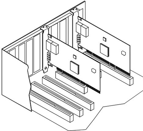
3. Push the adapter into the slot until the adapter is firmly seated, and then secure the adapter bracket with the screw you removed in step 2.
