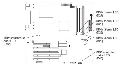
Each error LED turns on to indicate a problem with a specific component. After a problem is corrected, its LED will not turn on the next time the computer is restarted; if the problem remains, the LED will turn on again. See the "Solving problems" in the *User's Guide* on the IBM *IntelliStation Documentation* CD for additional information.
