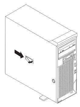
5. If you have not done so already, make sure that the two front stabilizing feet (if your model has rotating feet) are rotated outward so that they properly support the computer. Rotate each foot outward 90 degrees (see "Moving the stabilizing feet" on page 10).
