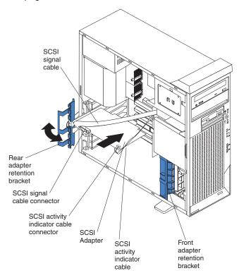
4. Complete the installation of the optional SCSI adapter.
