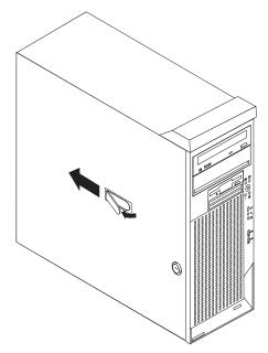
Attention: For proper cooling and airflow, replace the side cover before turning on the computer. Operating the computer with the cover removed might damage computer components.
