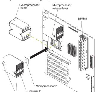
Complete the following steps to install an additional microprocessor.
