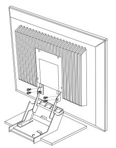
d. Remove the two screws that attach the lower cable cover to the bottom of the monitor; then, store the cable cover for possible future use.
