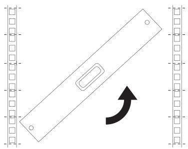
12. Attach the rear slide-rail brackets to the rack cabinet using four screws from the miscellaneous hardware kit.
