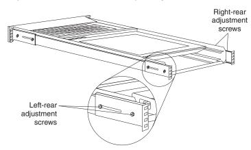
9. Tighten all four slide-rail adjustment screws.
