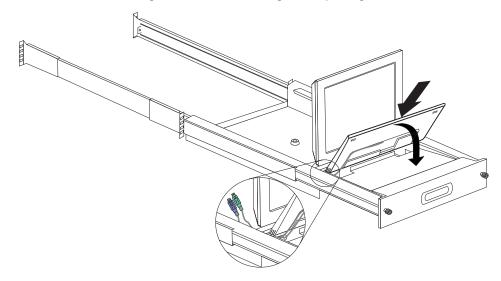
6. Route the keyboard and mouse cable toward the rear of the tray and beside the video and power cables; then, install the cable cover that you removed earlier.
