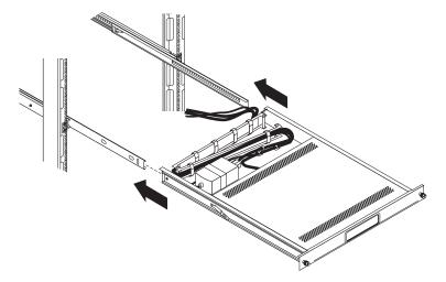
14. Press the release latches; then, push the flat-panel monitor and keyboard tray completely into the rack. There will be resistance initially as the ball-bearing assemblies align between the inner and outer rails. Pull the tray out halfway; then, push it back in to seat the tray in the rails. Do this a few times until the tray moves smoothly in the rails.
