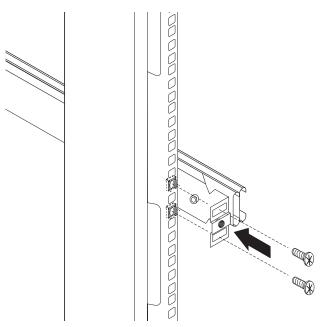
9. Loosely attach the back of the slide-rail brackets to the rack cabinet using four screws. Make sure that the slide-rail brackets extend outside of the rack-cabinet mounting flanges.
