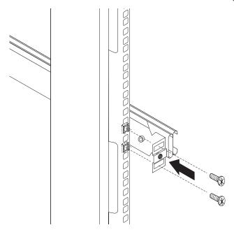
10. Loosely attach the back of the slide-rail brackets to the rack cabinet using four screws from the miscellaneous hardware kit. Make sure that the slide-rail brackets extend outside of the rack-cabinet mounting flanges.
