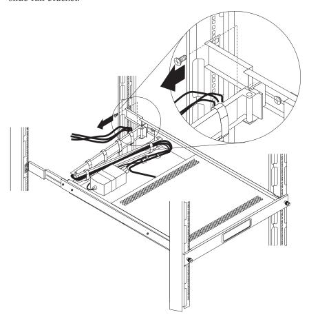
4. Fully extend the monitor and keyboard tray; then, temporarily remove the keyboard-and-mouse, video, and power cables from the cable-management arm.
