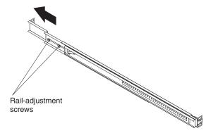
9. Adjust the outer slide-rail brackets to fit the depth of the rack cabinet; then, attach the front of the slide-rail brackets to the rack cabinet using four screws from the miscellaneous hardware kit. Make sure that the slide-rail brackets extend outside of the rack-cabinet mounting flanges.
