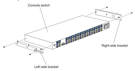
2. Install the console switch behind the flat-panel monitor and keyboard tray using two screws from the miscellaneous hardware kit.
