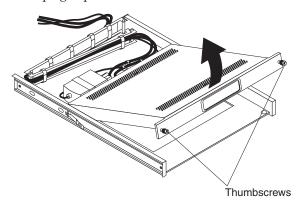
5. Carefully set the keyboard into the tray; then, route the keyboard-and-mouse cable through the cord clip on the bottom, up through the opening on the right side of the tray, and toward the cable-management arm. Pull the full length of the cable through the opening.
