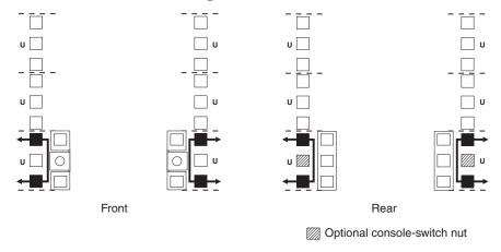
8. Loosen the two rail-adjustment screws on each of the outer slide rails; then, extend the rails to their maximum outward adjustment.
