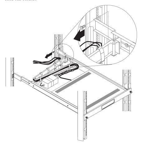
5. Fully extend the monitor and keyboard tray from the front of the rack cabinet; then, push in the release latch on each side of the tray and slide the monitor
