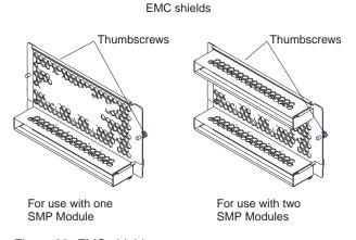
Figure 33. EMC shields
