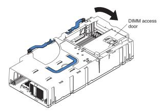
Figure 36. Opening the DIMM access door
