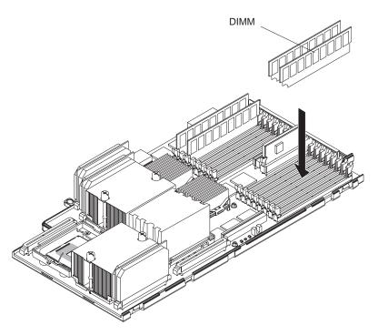
Figure 35. DIMM installation
