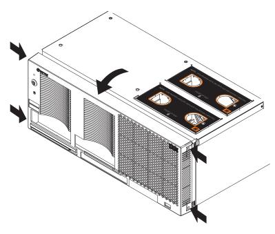
Figure 10. Removing the bezel
