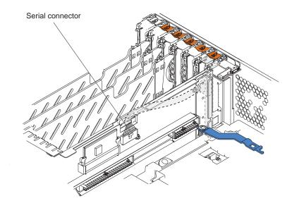
Figure 20. Route the serial port ribbon cable through the slot
