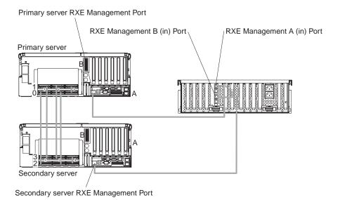
Figure 71. Cabling an RXE Management Port - 16-way configuration
