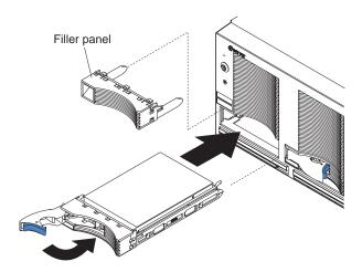
Figure 21. Installing a hard disk drive
