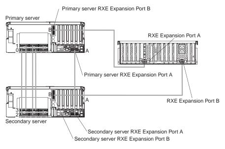
Figure 68. RXE Expansion Port cabling in a 16-way configuration
