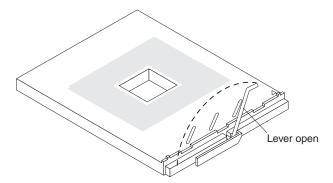
Figure 46. Microprocessor locking lever fully open
