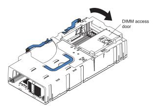
Figure 40. Opening the DIMM access door
