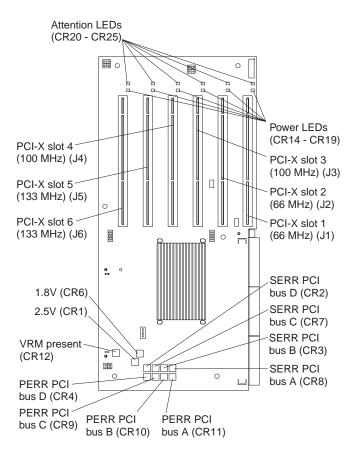
Figure 6. PCI-X board connectors and LEDs
