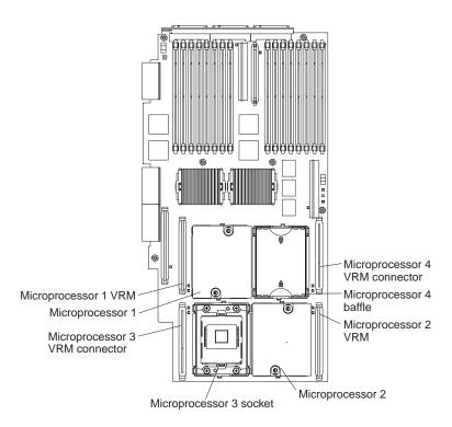
Figure 42. Microprocessor connector and component locations
