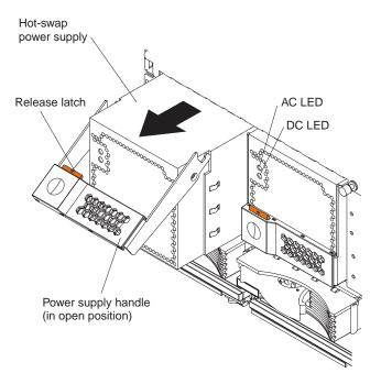
Figure 12. Removing a power supply
