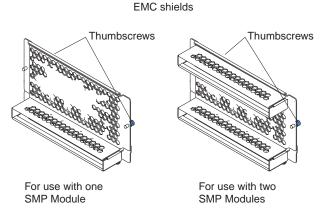
Figure 25. EMC shields
