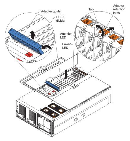
Figure 18. PCI-X slot components
