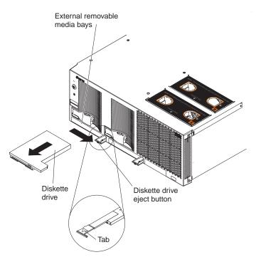
Figure 22. Installing a diskette disk drive
