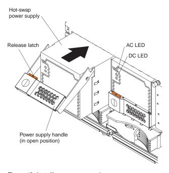
Figure 13. Installing a power supply
