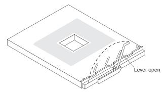
Figure 44. Microprocessor locking lever fully open
