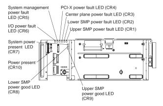
Figure 3. Center plane LEDs
