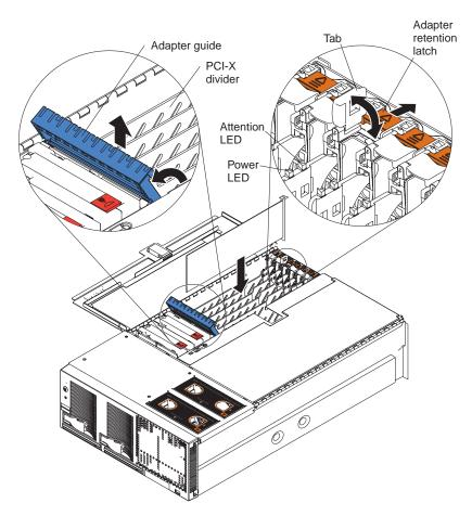
Figure 15. PCI-X slot components
