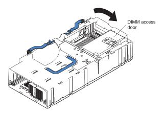
Figure 38. Opening the DIMM access door
