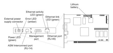
Figure 8. Remote Supervisor Adapter connectors and LEDs
