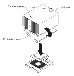
Figure 47. Aligning the heat sink over the microprocessor
