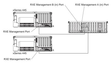
Figure 70. Cabling an RXE Management port - two stand-alone servers
