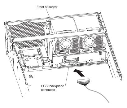
Figure 17. Connecting the SCSI cable to the SCSI backplane
