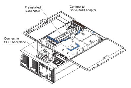
Figure 16. Location of preinstalled SCSI cable
