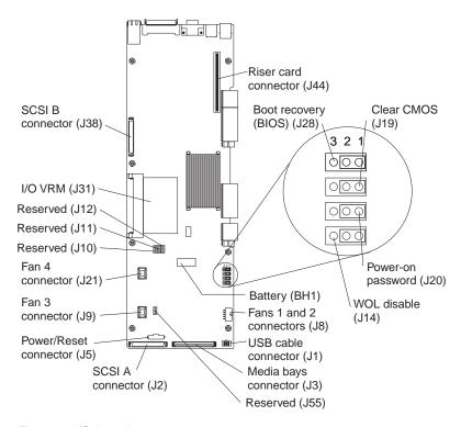
Figure 7. I/O board connectors
