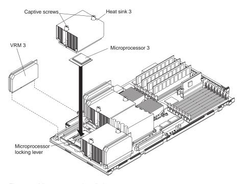
Figure 43. Microprocessor installation
