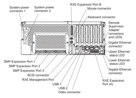
Figure 72. Rear view of xSeries 445
