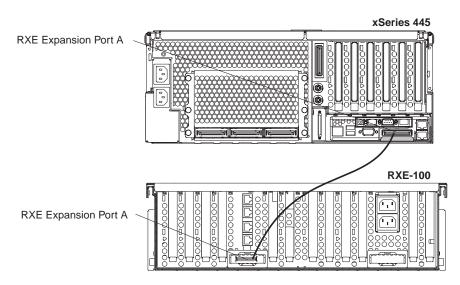
Figure 62. RXE Expansion Port cabling a server with one SMP Expansion Module
