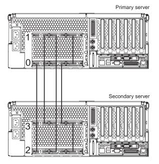
Figure 58. 16-way SMP Expansion port cabling
