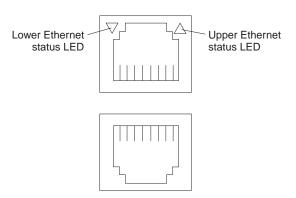
Figure 73. Gigabit Ethernet port
