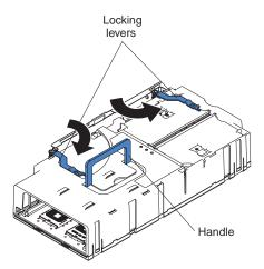
Figure 30. Locking lever position for installing the SMP Expansion Module
