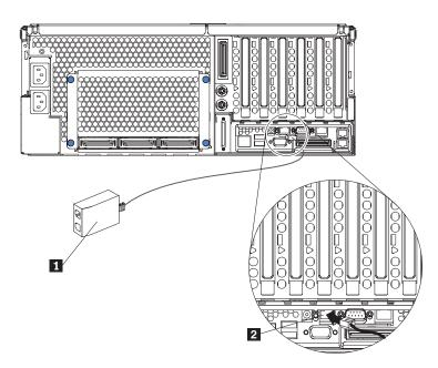
Figure 8. Connecting an ASM Interconnect module to an xSeries 445 server
