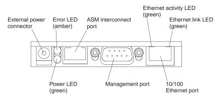
Figure 3. Remote Supervisor Adapter
