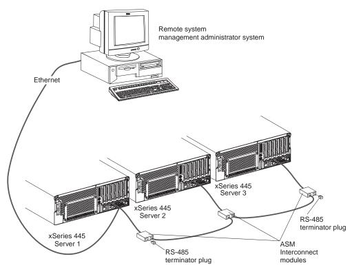
**Note:** The ASM Interconnect module is connected to the RS485 port on the back panel of the Remote Supervisor Adapter in each server.
