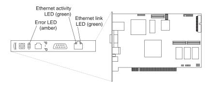
Figure 4. Ethernet LEDs locations on the Remote Supervisor Adapter
