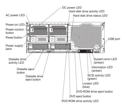
Figure 1. Front view of xSeries 445
