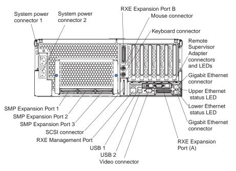
Figure 2. Rear view of xSeries 445
