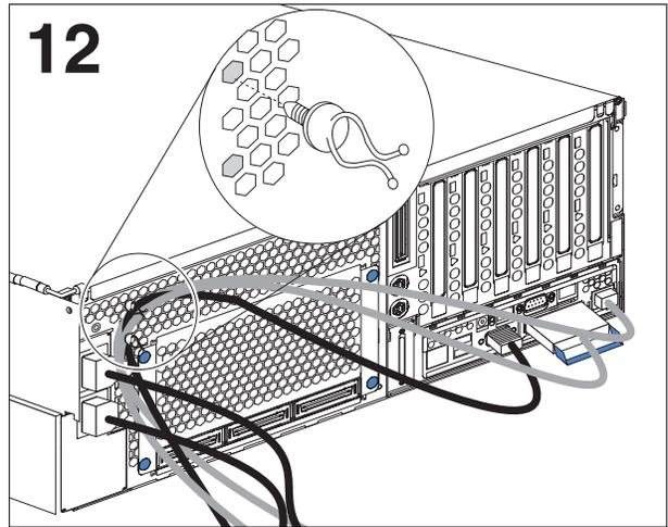
Attach cables to the rear of the server (such as keyboard, mouse, and monitor cables if required). Route the cables toward the left side of the server. Use cable clamps to secure cables along the way. Insert clamps only in the column of ventilation holes immediately to the right of the ac power connectors. If you insert the clamps in columns elsewhere, they will interfere with the removal of internal components.
