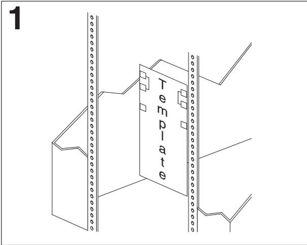
Use the attached rack mounting template to locate the holes on the front and rear rack mounting flanges.
