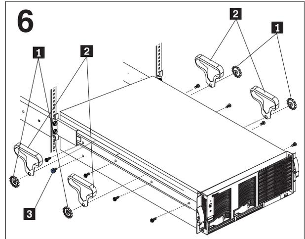
Use four M4 screws per side to secure the server to the rails; then, remove the rack-support wheels **1** and the handles **2** and store them in a safe place. Also remove the blue thumbscrew **3** from the left side of the server and store it in a safe place.
