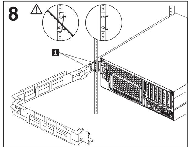
Press in on the slide-rail-locking latches and slide the server fully into the rack cabinet. Slide the cable-management-arm bracket over the right-rear M6 screws **1**. Ensure that both rear slide-rail brackets are vertically aligned; then, fully tighten the four rear M6 screws.
