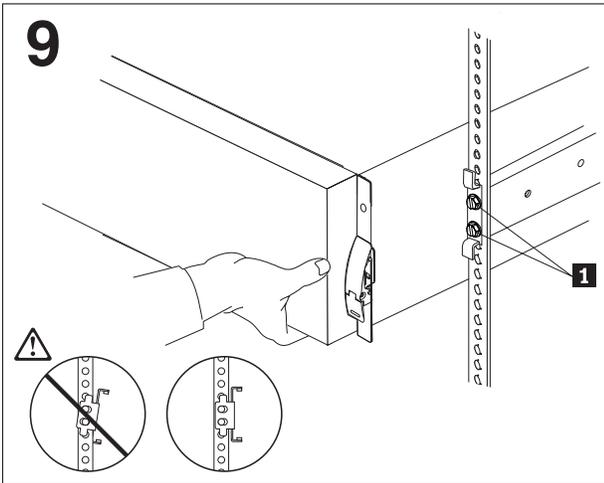
Slide the server halfway out of the rack cabinet; then, loosen but do not remove the four front M6 screws **1**. While one person supports the front of the server by lifting it slightly, ensure that the front slide-rail brackets are vertically aligned; then, fully tighten the four front M6 screws.
