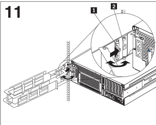
Slide the tab **1** on the cable management arm into the slot **2** in the hinge plate; then, release the hinge pins into the holes in the plate.
