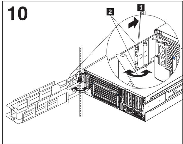
Slide the server fully into the rack cabinet until it locks in place. Using the handles **1** on the free end of the cable management arm, retract the spring-loaded hinge pins **2**; then, rotate the handles to lock the pins in the retracted position.
