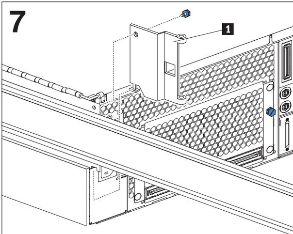
Insert the tab on the bottom edge of the cable management arm hinge plate **1** into the slot at the rear-left side of the server; then, attach the plate to the server with the M3.5 thumbscrew.
