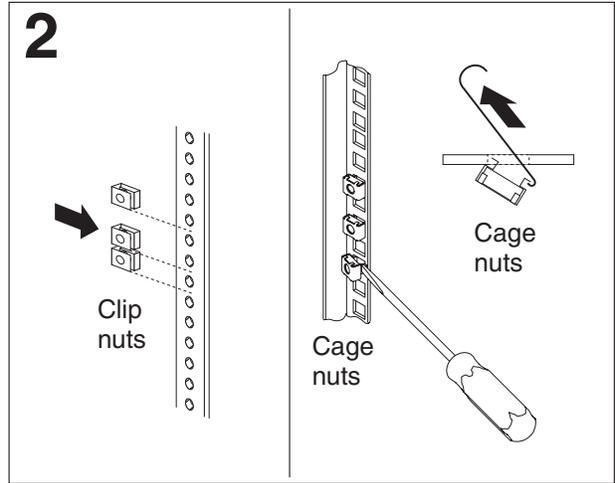
Install cage nuts or clip nuts as required for your rack cabinet. Use the cage-nut-insertion tool or a flat-blade screwdriver to install cage nuts.
