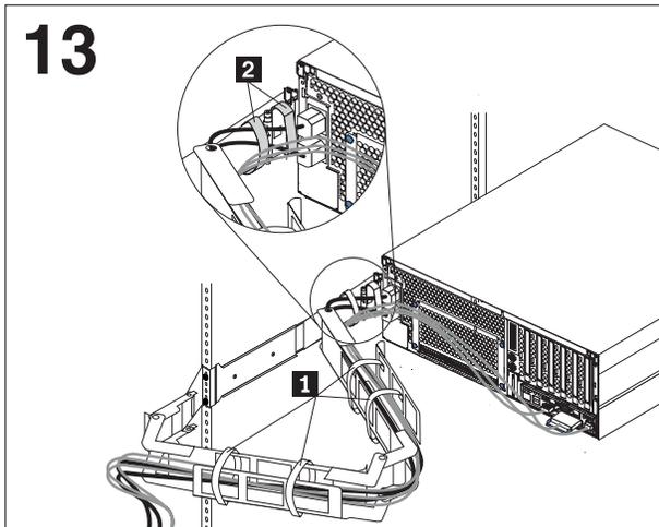
Route the cables through the cable-management arm, securing them with cable straps **1**. Use two cable straps **2** (one on each side of the hinge) to secure the power cords to the hinge plate.
