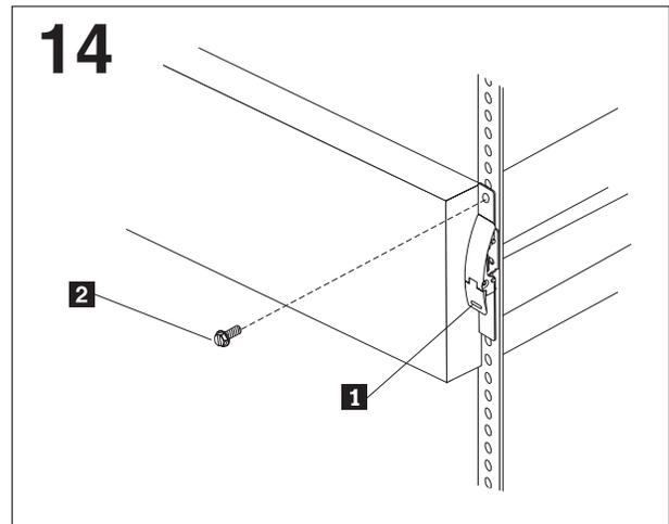
Slide the server into the rack cabinet until the release latches **1** lock into place.
