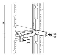
14. Install the screw that attaches the cable-management arm to the left slide-rail bracket; then, tighten all four slide-rail-adjustment screws.
