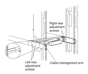
15. While one person pulls the tray halfway out of the front of the rack cabinet and supports the weight of the tray, attach the front of the tray to the rack cabinet using four of the screws from the miscellaneous hardware kit.
