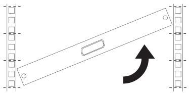
13. Adjust the rear slide-rail brackets to fit the depth of your rack cabinet; then, attach the brackets to the rack cabinet using four screws from the miscellaneous hardware kit.
