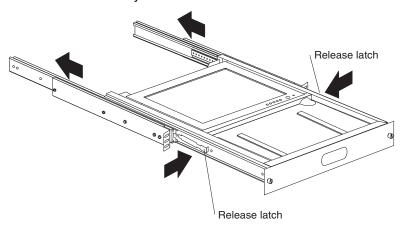
6. Remove the two screws per side that attach the remaining slide rail pieces to the tray; then, attach the corresponding new slide rail pieces to the tray using the same screws.
