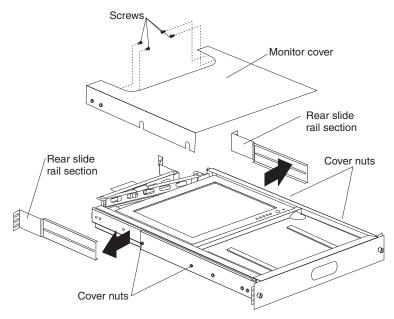
a. Remove the two screws on each side that attach the rear slide rail sections to the slide rail assembly.
