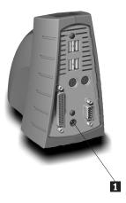
4. Connect one end of the two-foot USB cable to the computer USB connector and the other end of the cable to the USB cable connector on the front of the hub 2.
