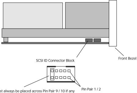
A jumper must always be placed across Pin Pair 9 / 10 if any SCSI ID other than the default (5) is selected.
