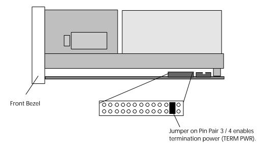
If the tape drive is the last device on the SCSI bus, the bus must be terminated at the drive. Some SCSI cables provide self termination and do not require terminators. To terminate the bus at the drive, attach a SCSI terminator (not provided) to the drive connector before attaching the SCSI cable.
