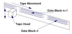
Figure 3. Longitudinal recording principles
