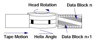
Figure 1. Helical Scan Principles
