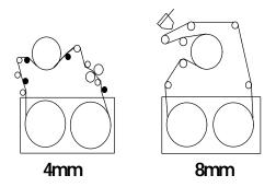
Figure 2. Helical scan tape paths
