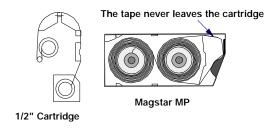
Figure 4. Longitudinal recording tape paths
