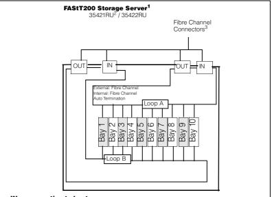
IN = connection to host **OUT** = connection to expansion units
