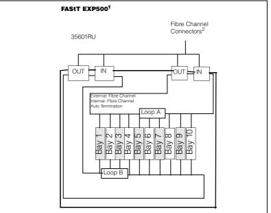
IN = primary or secondary (redundant) connection from FAStT500 Storage Server or previous FAStT EXP500 expansion unit daisy-chained from the storage server
