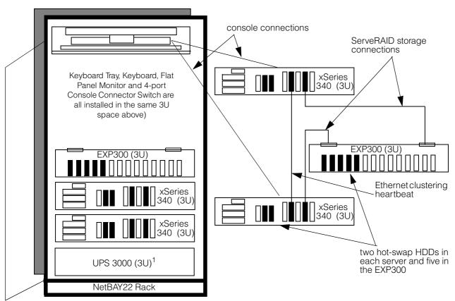
1. Either a UPS 3000 or PDU can be installed. Power options are not shipped standard with the cluster bundle. Power connections are not represented in this diagram.
