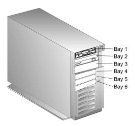
**Diskette Drive:** All models come with a 3.5-inch, 1.44 MB diskette drive in expansion bay 1 that uses 1 MB (unformatted) and 2 MB (unformatted) diskettes. For optimum use, format 1 MB diskettes to store 720 KB of data and 2 MB diskettes to store 1.44 MB of data.
