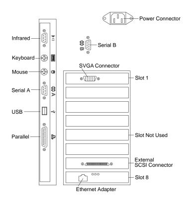
**Power Connector:** The server power cable attaches here.
