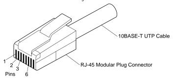
Table 6 shows the pin-number assignments for the RJ-45 Ethernet connector.
