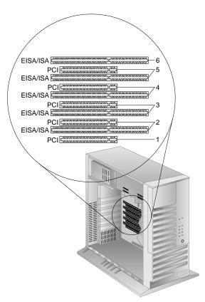
All PC Server 325 models have six expansion slots on the system board. Expansion slot 1 is PCI. Expansion slot 6 is EISA/ISA. The four remaining expansion slots (slots 2, 3, 4, and 5) are *shared expansion slots*. This means that you can install an adapter in either the PCI expansion slot or the adjacent EISA/ISA expansion slot, but not in both.
