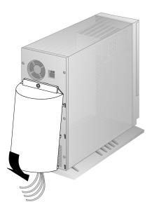
The security-cover option prevents the cables from being removed from the rear of the server, and prohibits other computers or devices from being attached to the unused connectors.
