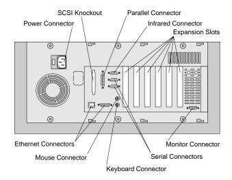
**Power Connector:** The server power cable connects here.
