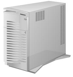
An example is the Model 3516 Hot-Swap Storage Expansion Enclosure, a mini tower that holds up to seven hot-swap hard disk drives. It is shipped without drives, so you must install at least one drive before you attach the enclosure to the server. To connect the enclosure to the external SCSI-2 connector on the server, you need a 68-pin to 68-pin external SCSI-2 cable.
