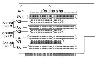
The PCI bus operates at up to 33 MHz with a 32-bit data path. PCI connectors support both 3.3-volt and 5-volt adapters. A separate power cable connects to the back of the riser card to supply 3.3-volt power.
