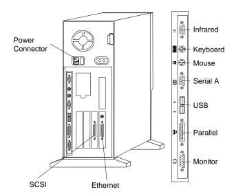
**Power Connector:** The server power cable attaches here.
