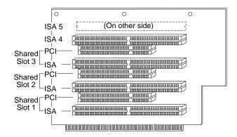
The riser card contains five industry standard architecture (ISA) expansion slots and three peripheral component interconnect (PCI) expansion slots. The three PCI slots and their adjacent ISA slots are shared expansion slots. You can install an adapter in either the PCI expansion slot or the adjacent ISA expansion slot, but not in both.
